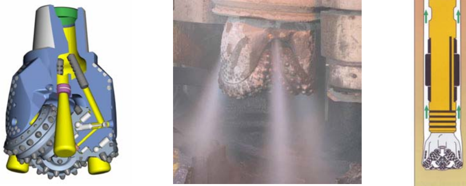
[fig15] - Air pathway through the nozzles and lugs; Flushing of the drill cuttings
