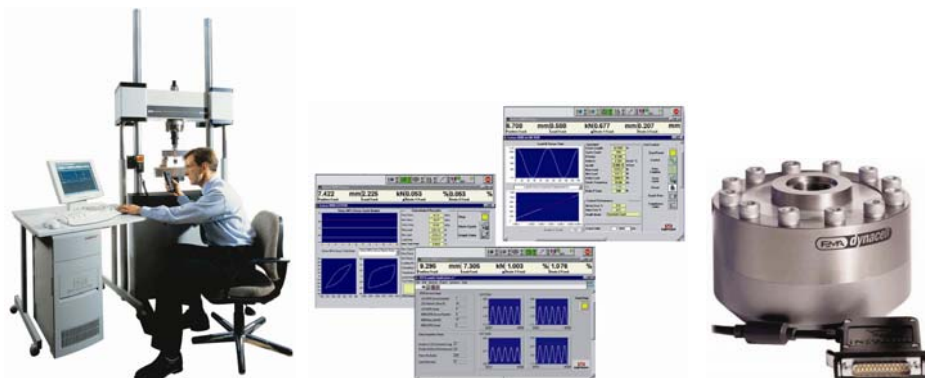
[fig26] - Fatigue test machine with controlling and data analysis software. Specifically designed load cell
