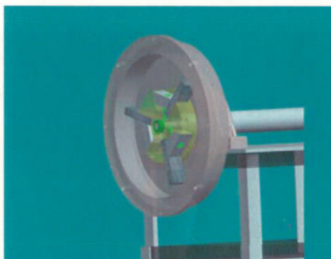
Figure 1. Three specimens are mounted on the impeller that rotates inside the hub. Hub is designed to hold 0.6 kg (1.3 lbs) of ore.
