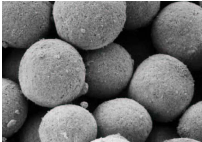
[fig3] - Electron microscope image of the agglomerates resulting from spray drying. Metal and carbide powder with a grain size of 1-3 \mu\text{m} was used, along with PEG (Polyethylene glycol) as press agent. The agglomerates average a 100 \mu\text{m} diameter [6] .
