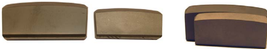
[fig5] - Dimensional comparison between green body and cemented carbide insert after sintering
