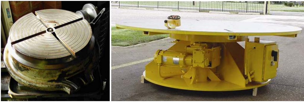
[fig41] – Rotary table hydraulically actuated and turntable for centred loading.
