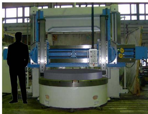
[fig32] – Vertical lathe with rock and silhouette as dimensional reference
