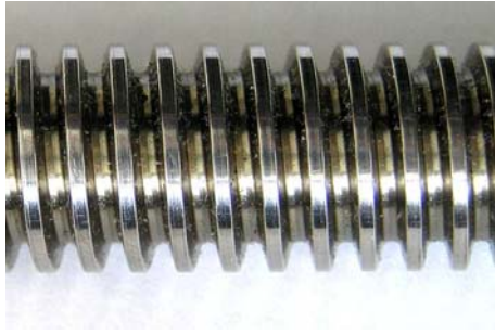
[fig36] – Acme thread used to guide and move the tool holder in vertical lathes
