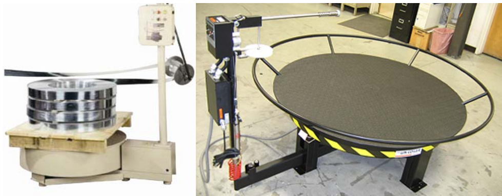
[fig42] - Depalletizer – a turntable used in uncoiling applications
