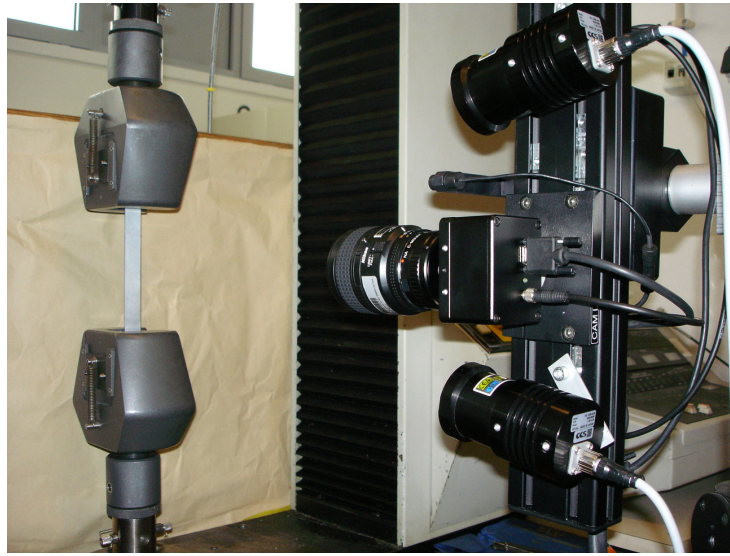
Figure 6.4: Off-axis tension test setup with low speed DIC data acquisition system.
