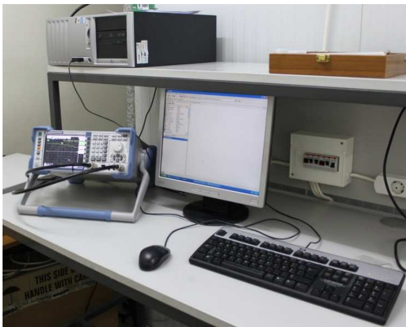
Figure 3.11 - Network analyzer and computer which controls rotating platform
