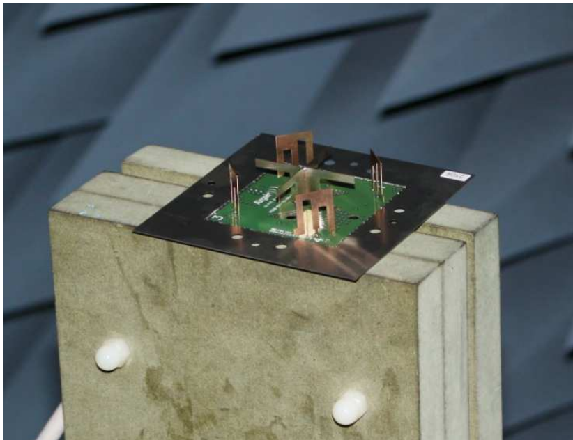
Figure 3.15 - Switched beam antenna without plastic box over the rotating platform
