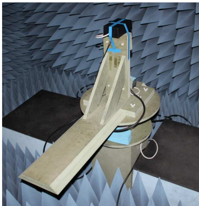
Figure 3.13 - Switched beam antenna to be tested over the rotating platform
