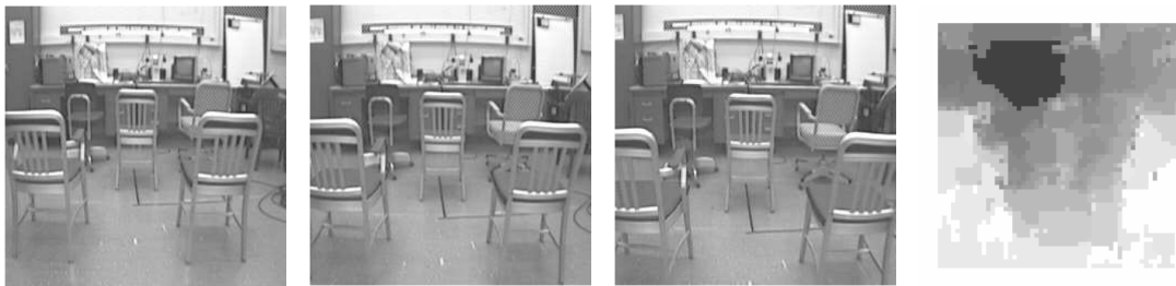
Figure 2.7: Example of an Optical Flow intensity extracted from a test sequence, from [4].
