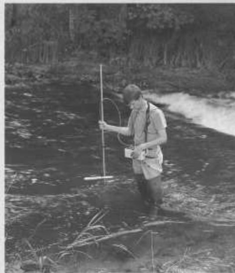
NAUTILUS velocity sensor, fixed on wading rod 20 mm dia. and HERES relocating device.
