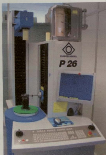
Figure 14 - KLINGELNBERG measuring machine.
