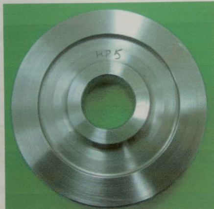
Figure 8 - Face without foundry defects.
