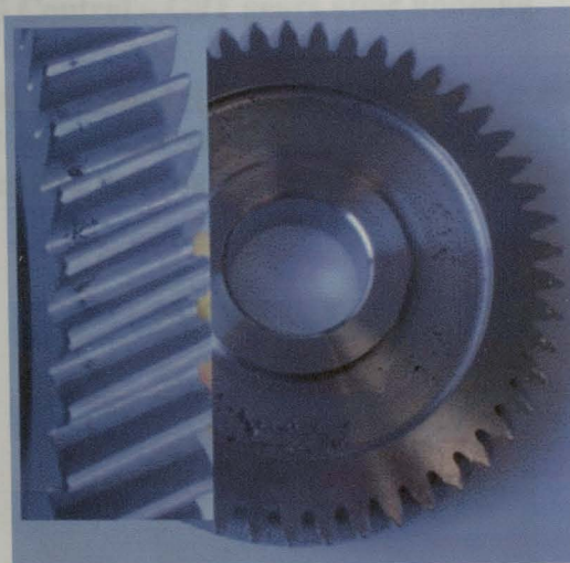
Figure 11 – Gear HP5 with foundry defects.
