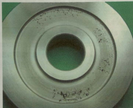
Figure 9 - Face with foundry defects.
