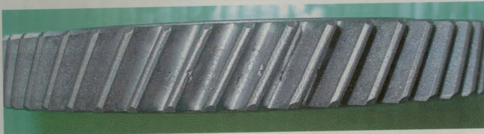
Figure 19 - Gear HP3 (M1D z49 left) after heat treatment, with foundry defects.
