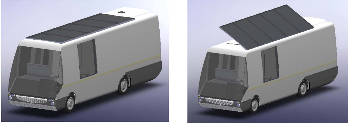
Figure 7-6: Solar panels orientation.
