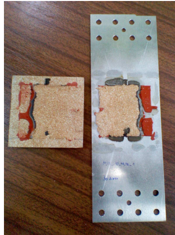
Figure 47- Cohesive rupture in the ceramic and cohesive rupture in the silicone at the opposite load edge for mixed adhesive joints
