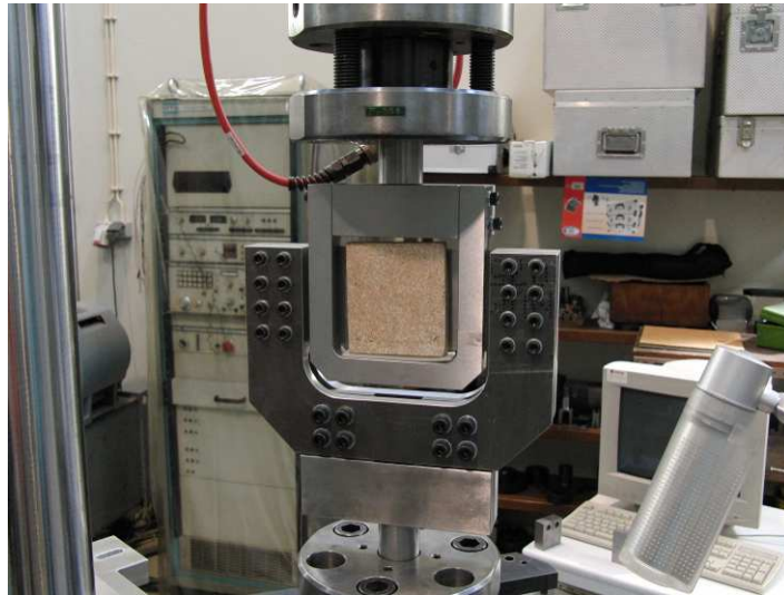
Figure 27 – Shear test in the MTS machine
