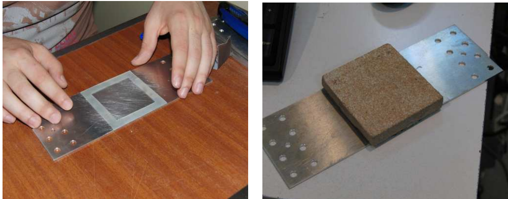
Figure 17 – Silicone to ensure the thickness and bond area to the specimen used for the mechanical experiments
