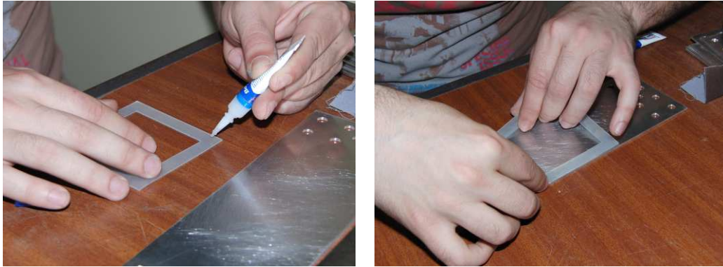
Figure 20 – Silicone square bonding
