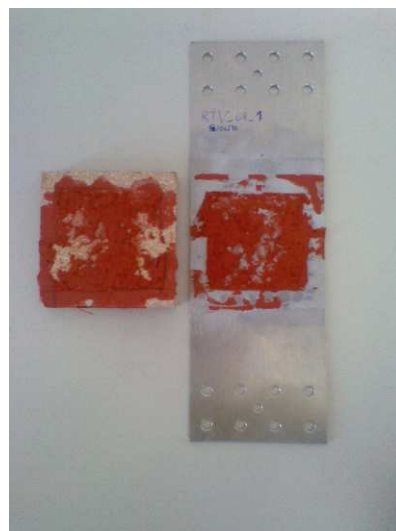
Figure 41- Cohesive fracture in the adhesive for an aluminium- ceramic joint with silicone
