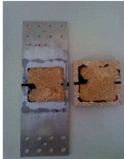
Figure 44 –Cohesive rupture in the ceramic for aluminium- ceramic joints bonded with the epoxy adhesive
