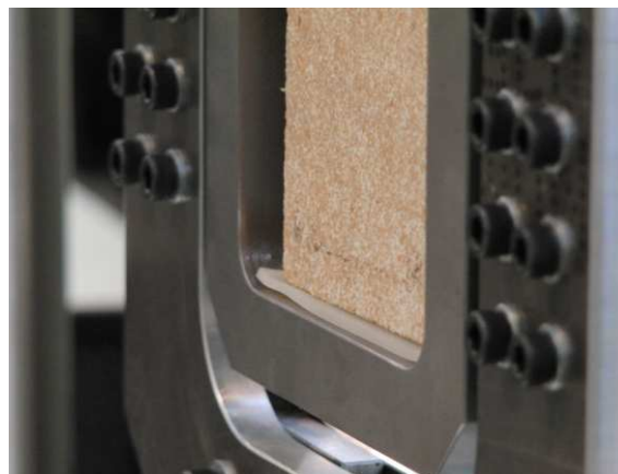
Figure 28 –Silicone piece between the ceramic and the loading tool
