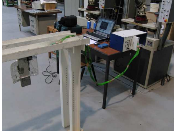
Figure 11 - Data acquisition system for temperature measurement
