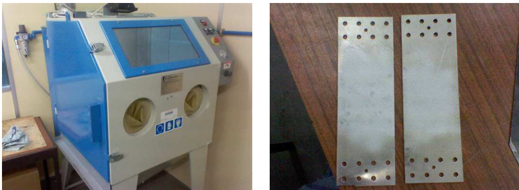
Figure 19 – Grit blaster used to treat the aluminium substrate
