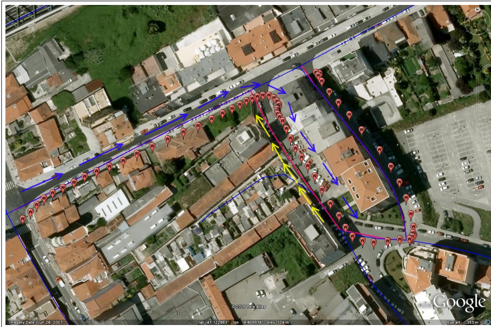
Figure 4.10: Detection of Wrong Direction - Results
