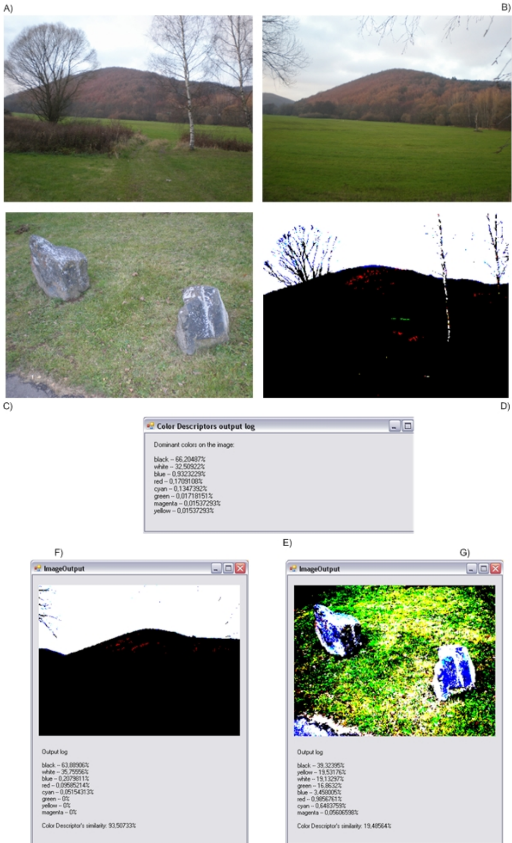
Figure 17: A) Query image B) Image from database C) Another image from database D) Colour descriptors' map from query image E) Colour features vector output from query image F) Similarity comparison results between query and the image on B) G) Similarity comparison results between query and the image on C)
