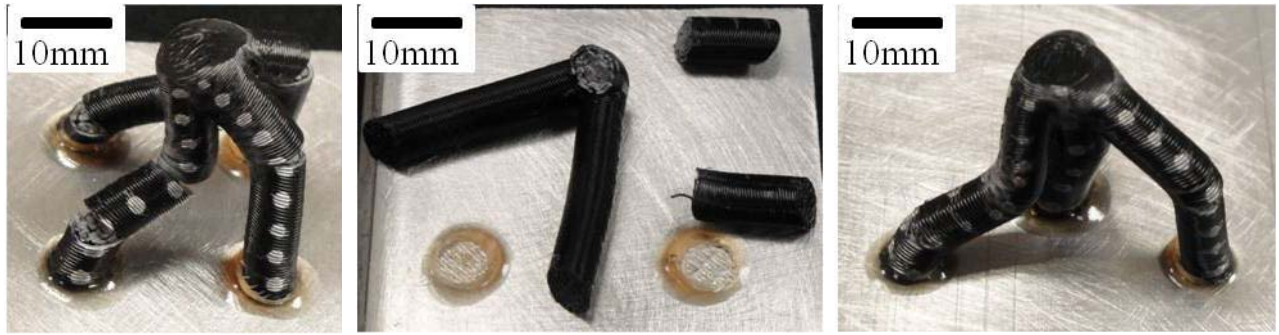
Figure 4.3 - Failed specimens after testing. From left to right: pyramidal, tetrahedral and SRT smallest topologies manufactured, with a height of 20.32mm.
