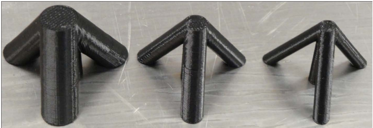
Figure 3.11 - Rapid prototyped SRT topology manufactured with different L/R ratios. From left to right: slenderness ratio of 5, 8 and 11 respectively.
