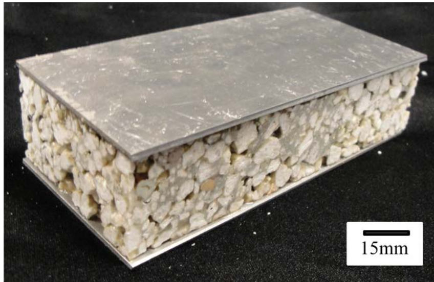
Figure 3.21 - 100mm long pumice/epoxy core bonded to 1.60mm thick aluminum facing sheets.
