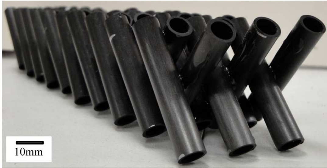
Figure 3.16 - Carbon tubes bonded together forming a two-dimensional lattice core.
