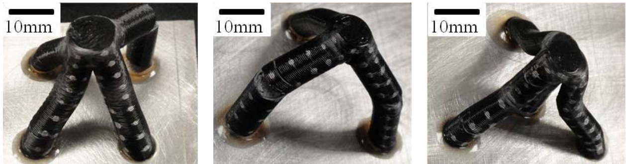
Figure 4.5 - Failed specimens after testing. From left to right: pyramidal, tetrahedral and SRT intermediate topologies, with a height of 25.40mm.
