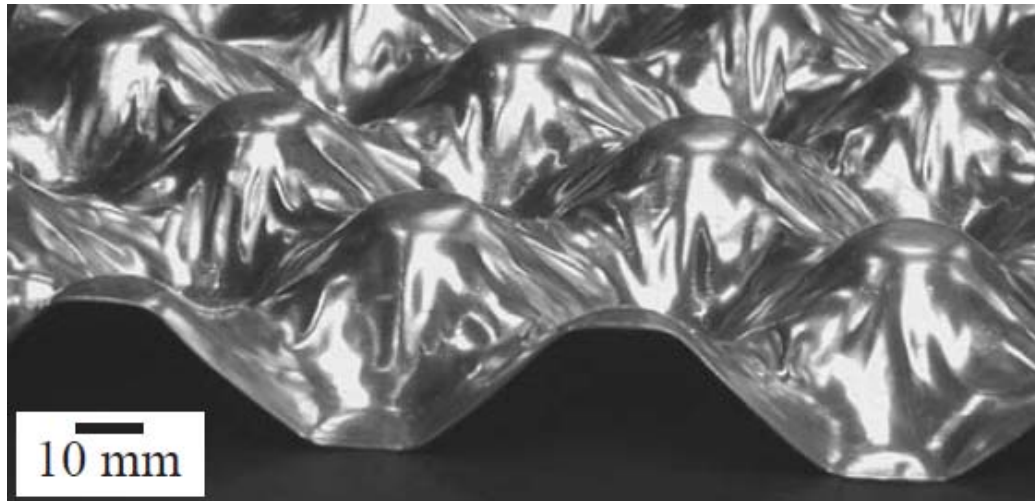
Figure 2.7 - Photograph of a cold formed aluminum egg-box used by Zupan et al [6].
