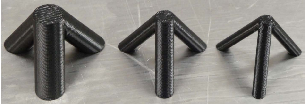
Figure 3.10 - Rapid prototyped Tetrahedral topology manufactured with different L/R ratios. From left to right: slenderness ratio of 5, 8 and 11 respectively.
