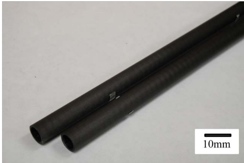
Figure 1.6 - Carbon fiber shafts. The manufacturing process is computerized and tightly controlled to meet strict tolerances in order to achieve properties consistency from shaft to shaft.
