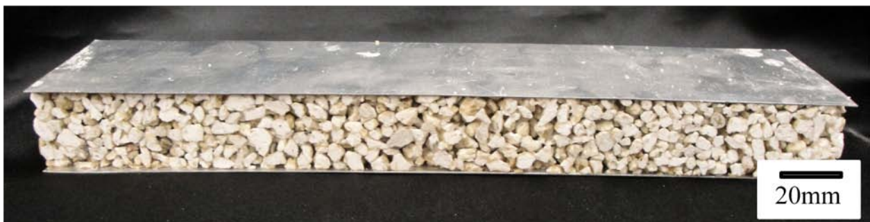
Figure 3.20 - 250mm long pumice/epoxy core bonded to 0.35mm thick aluminum facing sheets.
