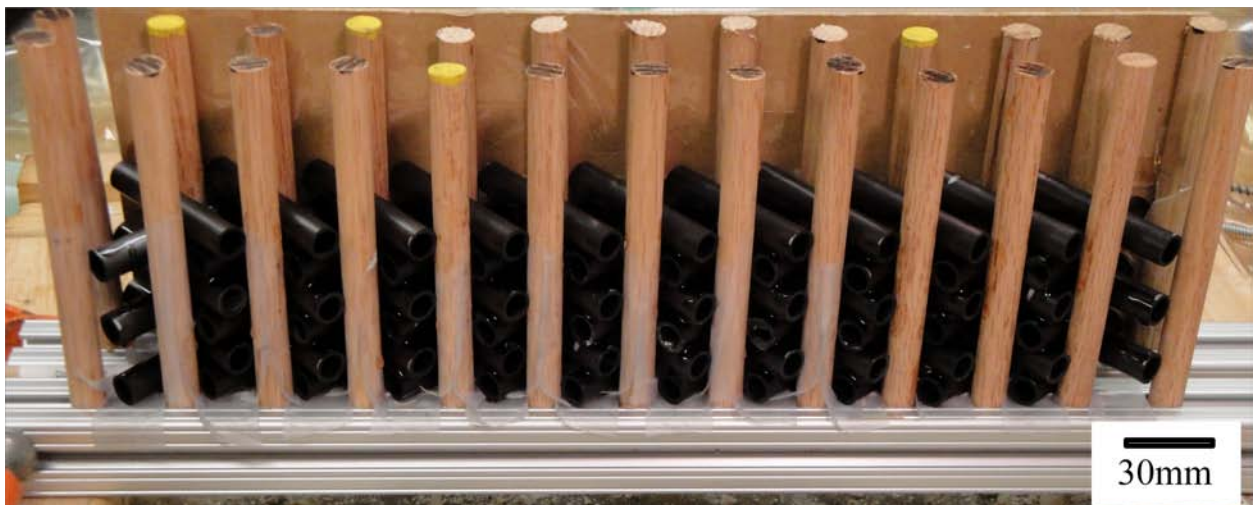
Figure 3.15 - Carbon tubes bonded with epoxy and displaced between the dowels at a 45 degree angle. A coat of epoxy is applied between each layer of tubes to ensure proper bonding in the contact points.
