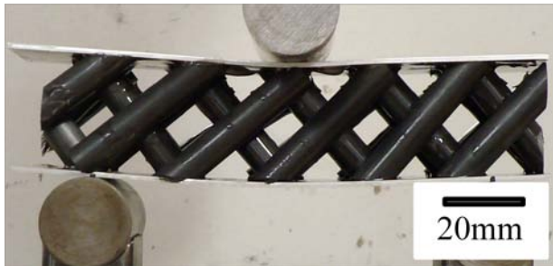
Figure 4.18 - Images of the specimen with a relative density of 0.174 with the thicker face sheets in the beginning of the test (top) and ending (bottom).
