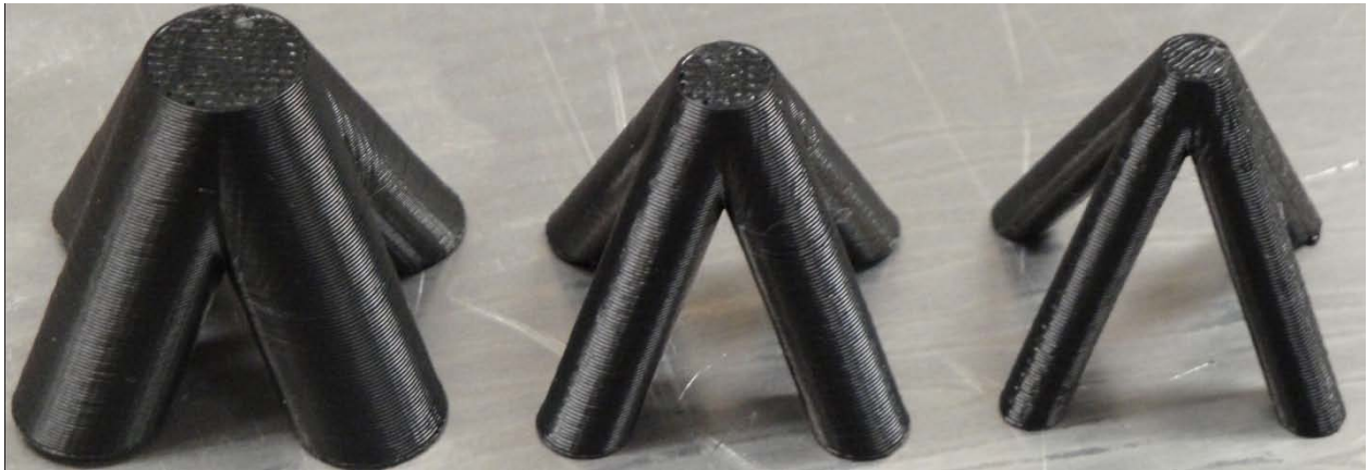
Figure 3.9 - Rapid prototyped Pyramidal topology manufactured with different L/R ratios. From left to right: slenderness ratio of 5, 8 and 11 respectively.
