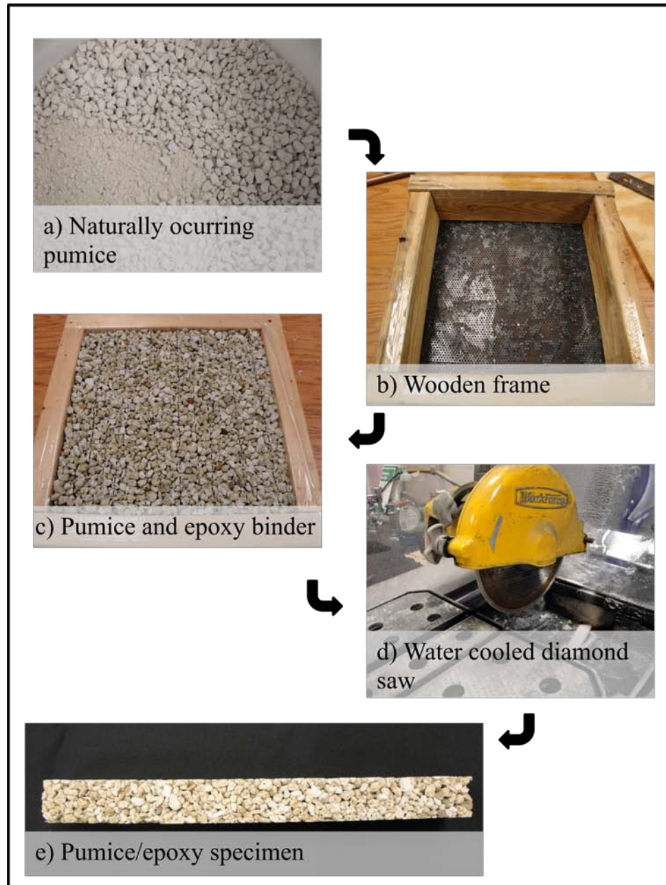
Figure 3.19 - Flow chart of pumice/epoxy specimen preparation. Pumice is provided in its naturally occurring state. A wooden frame is assembled with a bottom perforated plate to enable excess binder to flow out of the panel. The frame is then filled with pumice and binder is poured evenly on the panel. When the binder sets a diamond saw is used to cut specimens with the desired dimensions.
