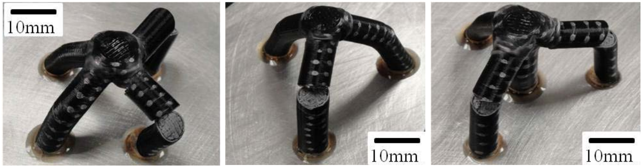
Figure 4.7 - Failed specimens after testing. From left to right: pyramidal, tetrahedral and SRT largest topologies, with a height of 30.48mm.
