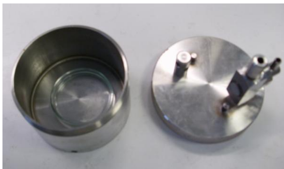
Figure 9 Petri dish inside the metal cylinder (9 cm inner and 10 cm outer diameter)
