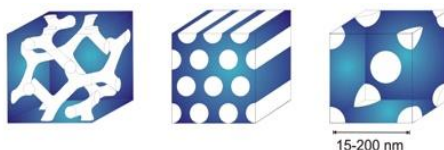
Figure 5 Examples of the types of nanoporous polymers realized by the Nanoporous Group
