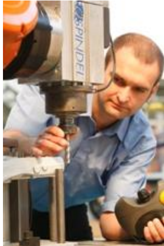
Figura 1.17 - Operador a utilizar a técnica "lead-to-teach" ( http://www.abb.com/cawp/seitp202/df84fb365192587a482573b00025d109.aspx )
