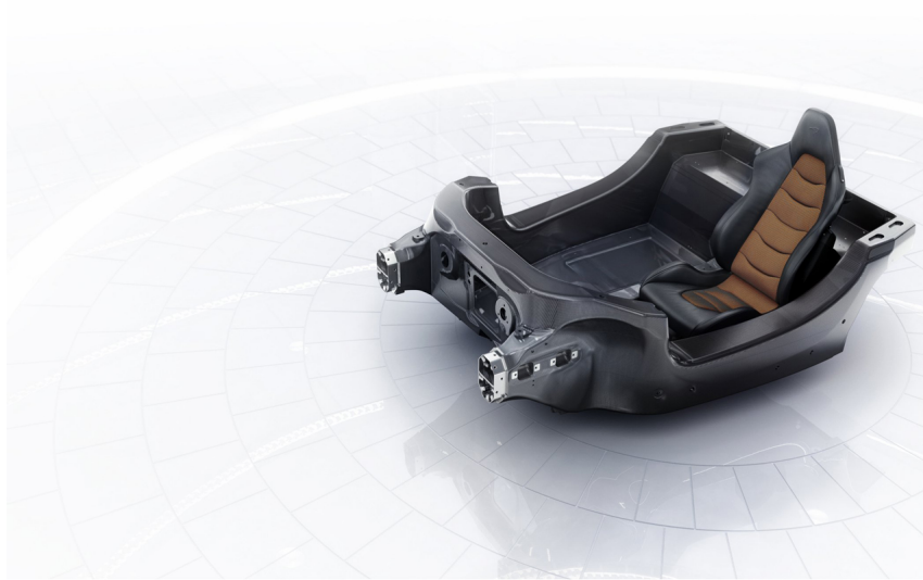
Figure 1.1: Carbon fiber chassis as an example for future piezoelectric transducers integration for vibration control.
