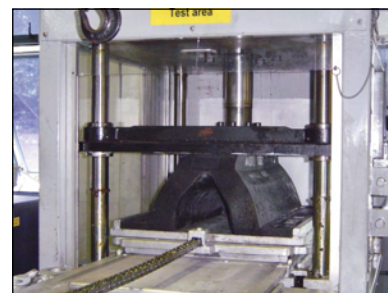
Speed testing of AN fender
