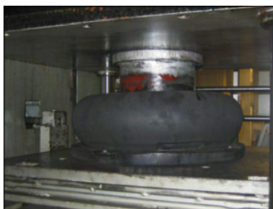
Fatigue testing of SCN fender
