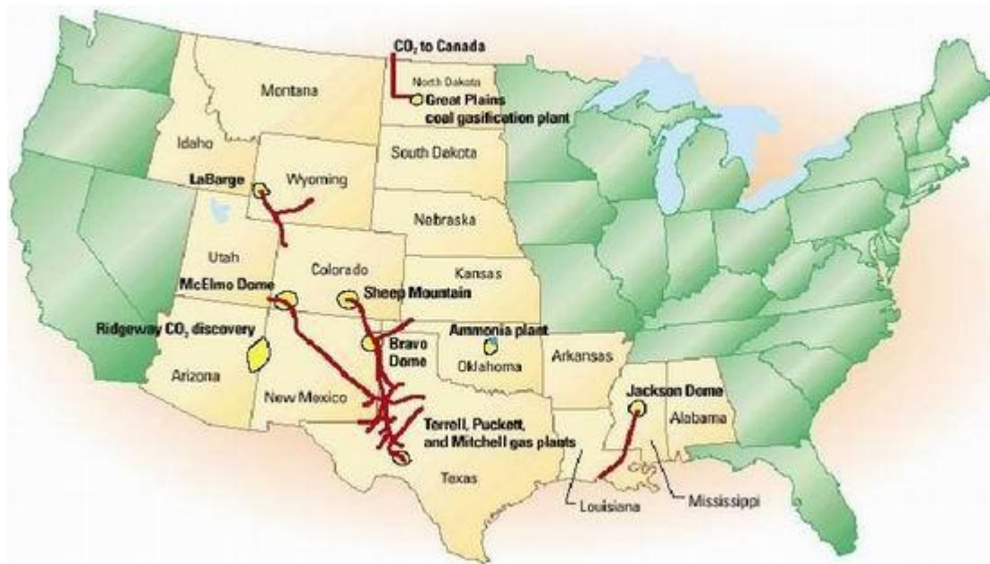
Figure 3. CO 2 pipelines in the USA. [17]
