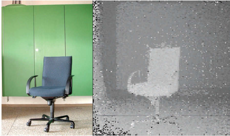
Figure 8. - An office chair (left) and as viewed by a SR4000 sensor (right).
