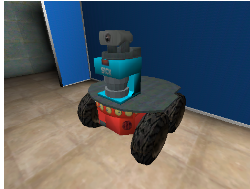
Figure 21. - Image of the original P2AT in USARSim, the robot modified to be used for testing.
