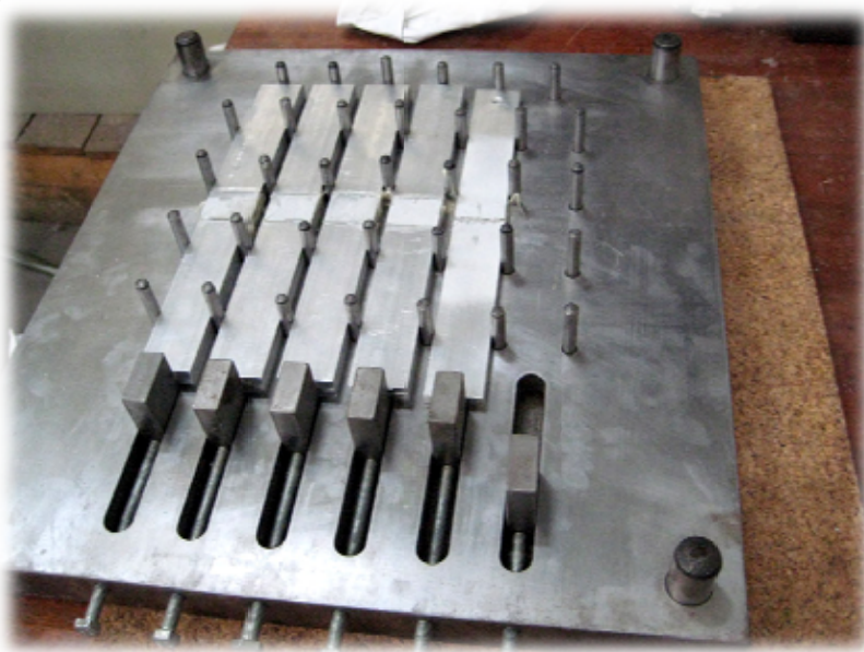
FIGURE 17 -MOULD USED TO PRODUCE SINGLE LAP JOINT SPECIMENS
