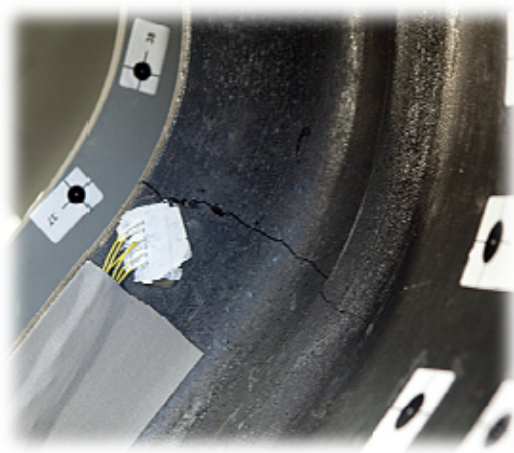
FIGURE 4 - DAMAGED CARBON-CARBON PANEL (18)
