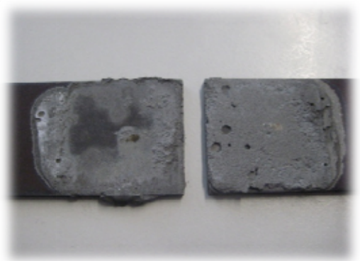
FIGURE 19-FRACTURE SURFACE OF SINGLE LAP JOINT SPECIMENS (1/2)
