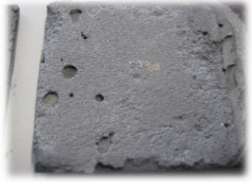
FIGURE 20-FRACTURE SURFACE OF SINGLE LAP JOINT SPECIMENS (2/2)
