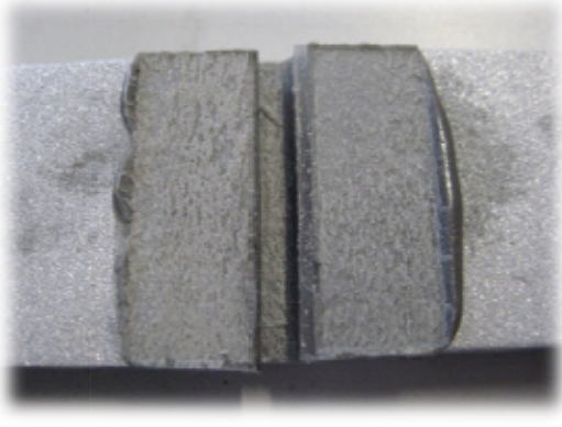
FIGURE 36- AV138 90 DEGREES TAPER FRACTURE SURFACE
