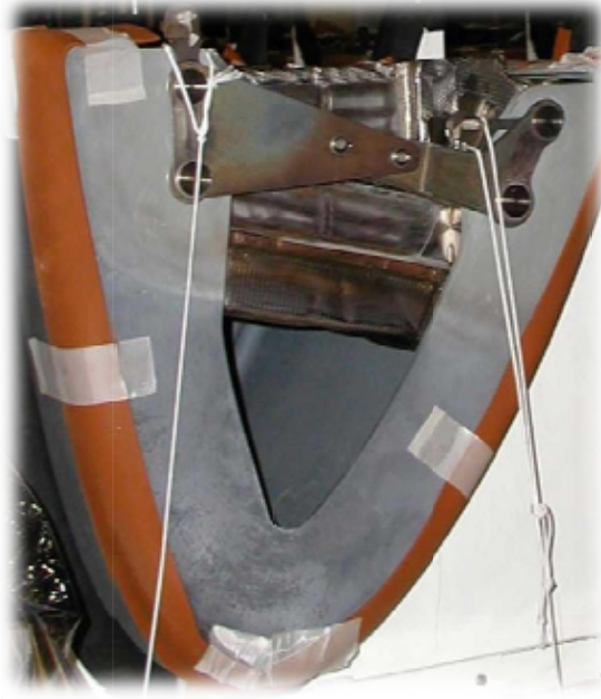
FIGURE 8 - CARBON-CARBON PLATE MOUNTED IN TITANIUM INSERT (18)
