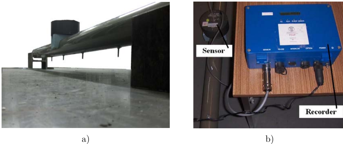
Figure 5.35: a) Photo of the experimental setup; b) accelerometer and recorder used in the experiment
