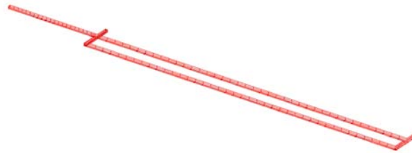
Figure 2.39: FE mesh for the reinforcement
