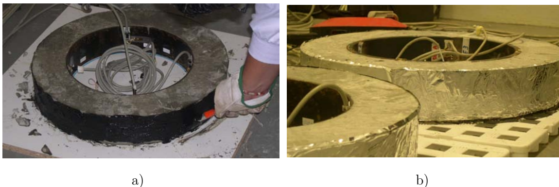
Figure 5.19: a) Application of the bituminous paint on the external surface of the concrete ring; b) Experiment after sealing and placement over final support system
