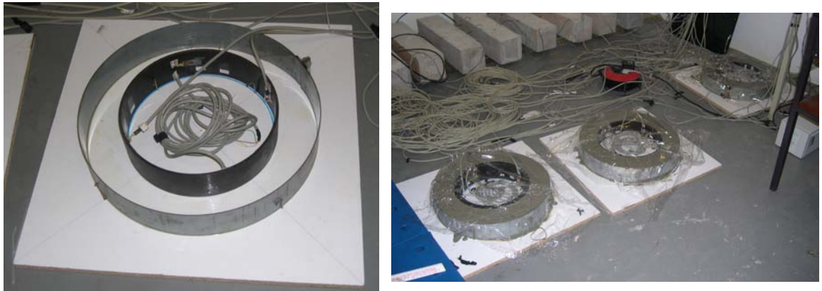
Figure 5.18: Appearance of the restrained ring test: a) before casting; b) after casting
