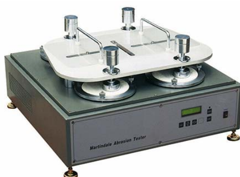
Figure 3.17. Martindale abrasion tester [154].
