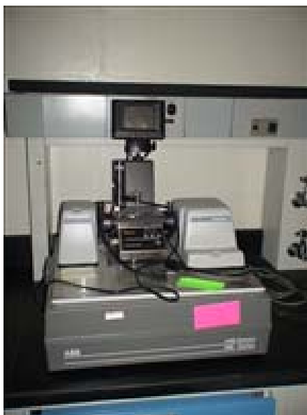
Figure 3.13. FTIR BOMEN (model MB 104).
