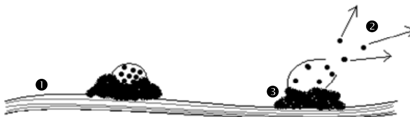
Figure 2.1. Schematic representation of the release of the active agent on the skin. 1. Textile fibre; 2.Release of the active agent on the skin; 3.Binder.
