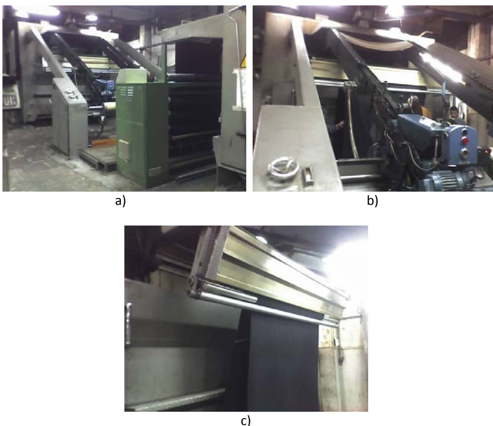
Figure 3.3. Several views of the industrial Foulard during the impregnation process of scented microcapsules. a) Overview of the Foulard; b) View of the fabric entry in the oven for the thermofixing and curing steps. c) View of the output of the final fabric with impregnated microcapsules.
