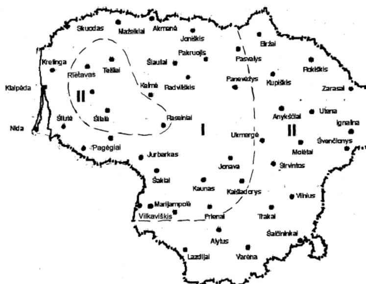
Fig.2.9- Lithuania snow load areas. Image of Statybus Techniniai Reglamentai (Construction Technical Regulations of Lithuania)
