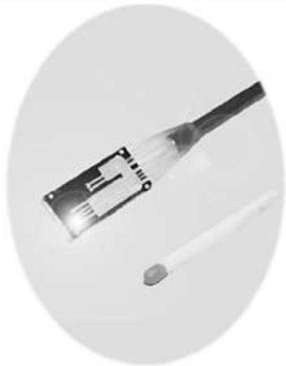
Fig. 9- O2C sensor containing 6 fiber glass elements 80
