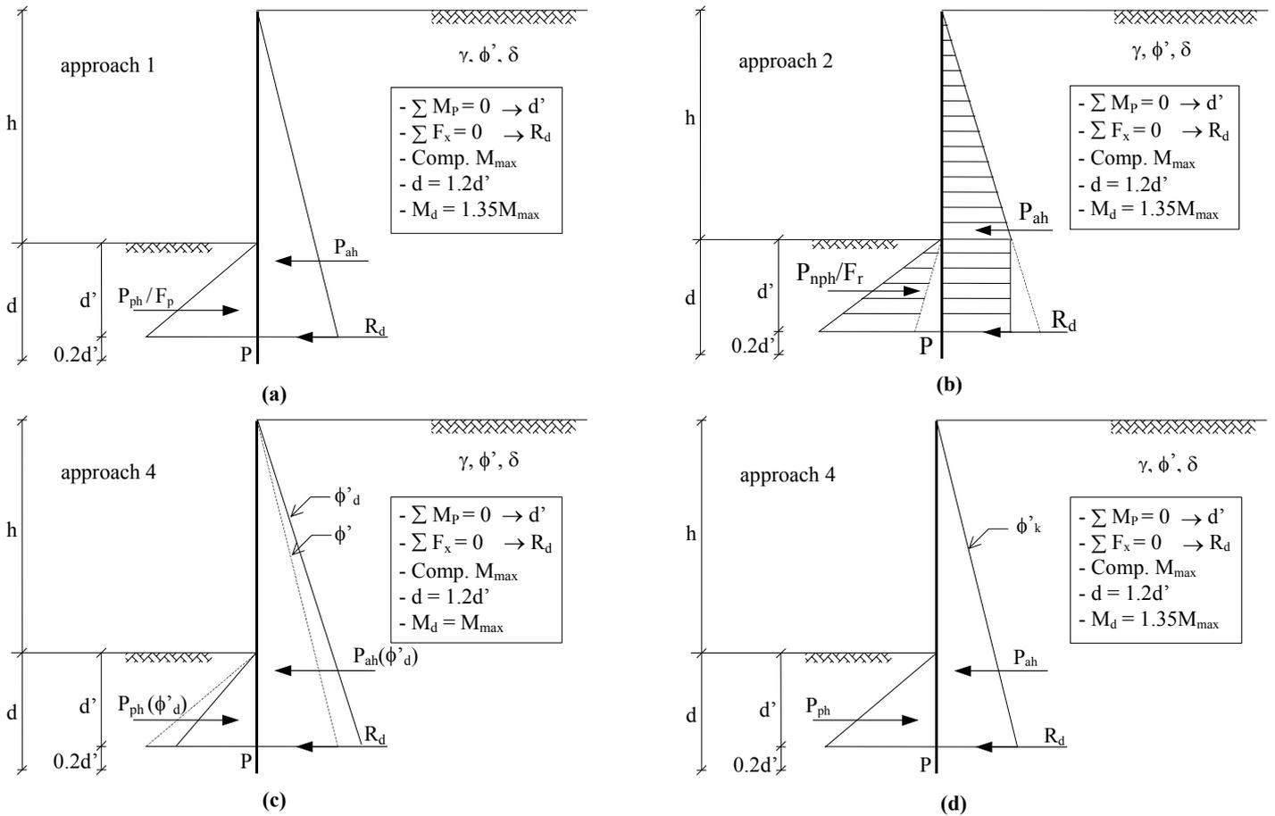
Figure 2. Approaches for the introduction of safety in the design of flexible cantilever retaining walls: (a) dividing the passive thrust by  $F_p$ ; (b) dividing the net passive thrust by  $F_r$ ; (c) EC 7 - Case C; (d) EC 7 - Case B
