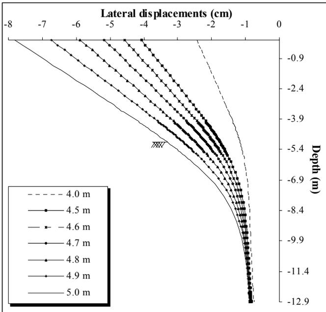
Figure 5. Wall designed according *approach 2* (W.L.1,  $\delta = (2/3) \phi'$ ): evolution of the lateral wall displacements
