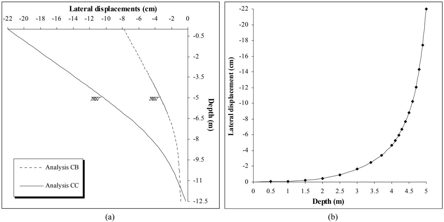
Figure 9. Lateral wall displacements (W.L.1,  $\delta = (2/3) \phi'$ ): (a) final distribution from analyses CB and CC; (b) - evolution of the displacement of the top of the wall with the current excavation depth in analysis CC
