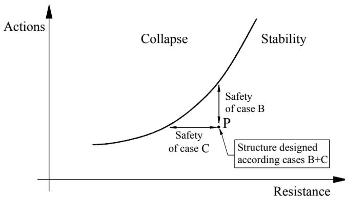
Figure 8. Scheme of safety checks for the Cases B+C approach of EC 7
