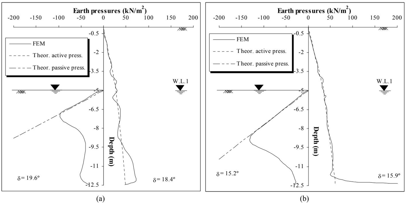
Figure 10. Effective final normal earth pressures on both sides of the wall (W.L.1,  $\delta = (2/3) \phi'$ ): (a) - analysis CB; (b) - analysis CC
