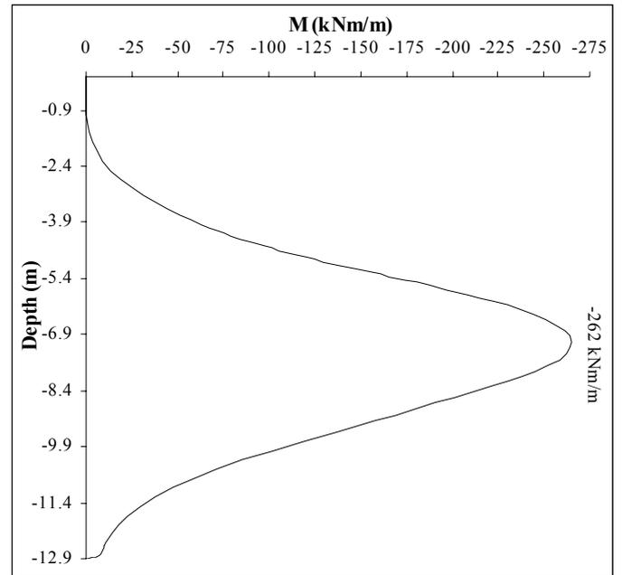
Figure 6. Wall designed according *approach 2* (W.L.1,  $\delta = (2/3) \phi'$ ): distribution of the final wall bending moments
