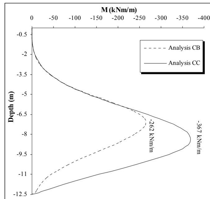
Figure 11. Distribution of the design wall bending moments (W.L.1,  $\delta = (2/3) \phi'$ ) from analyses CB and CC
