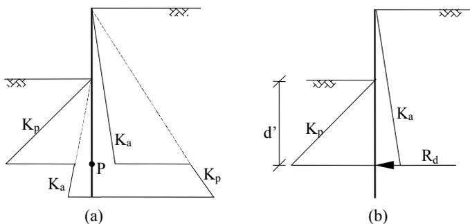
Figure 1. Limit equilibrium method of design: (a) - idealized distribution of earth pressures on the wall; (b) - system considered in the equilibrium equations.
