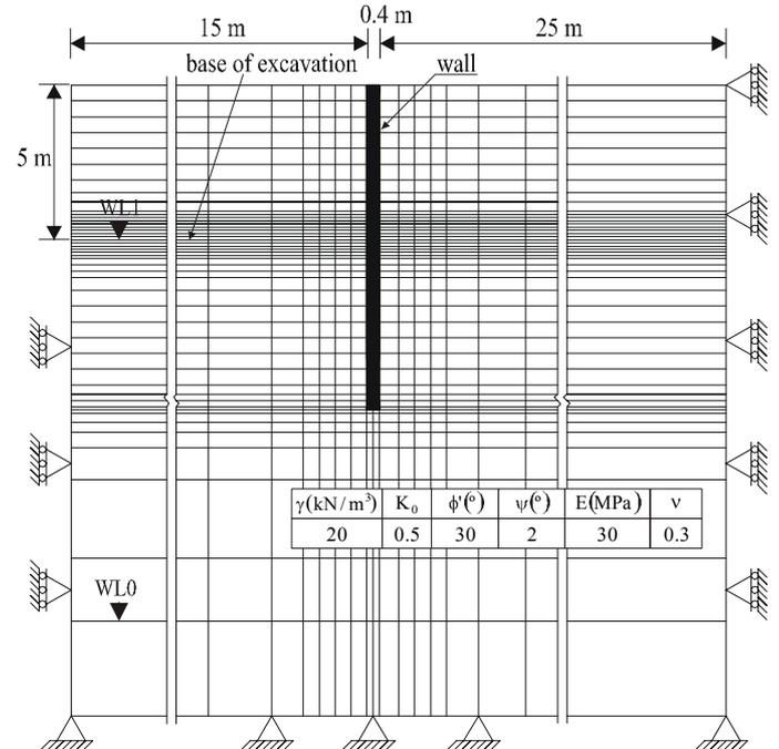
Figure 4. Finite element mesh and main assumptions of the numerical case study
