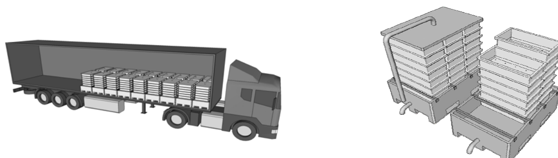
Figure 5.3 Illustration of prototype boxes to accommodate crabs from the fishing vessel to holding facilities (adapted from the EU Collective Research CRUSTASEA project).
