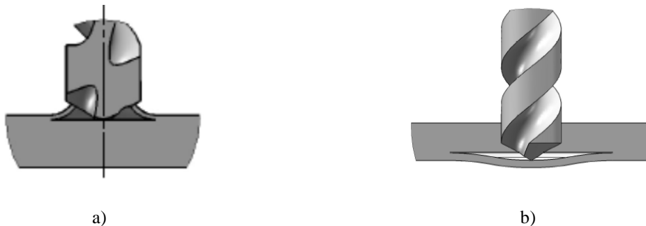
Figure 1 Delamination mechanisms: a) Peel-up; b) Push-down.
