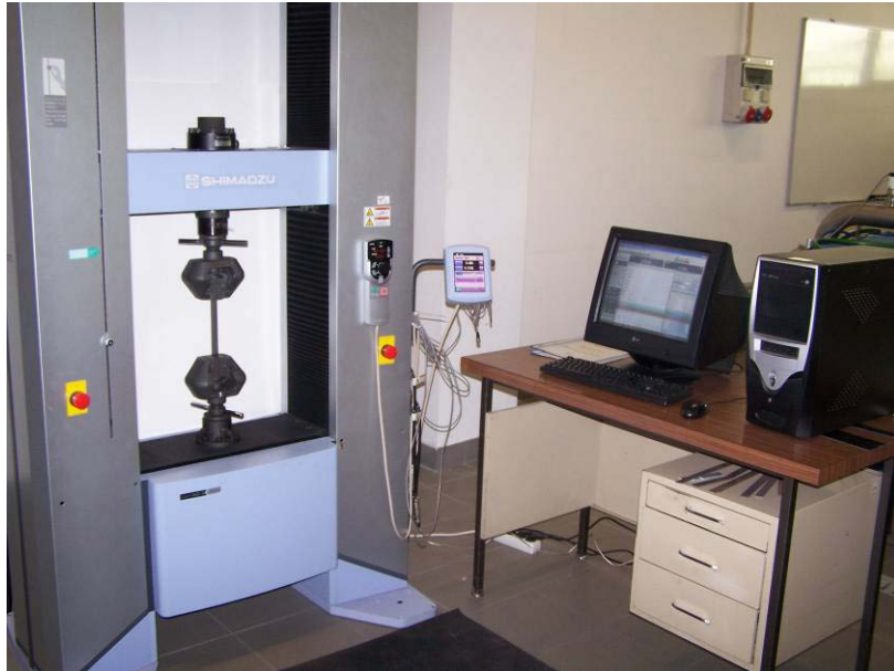
Figure 5 Mechanical test setup: Open-hole tensile strength
