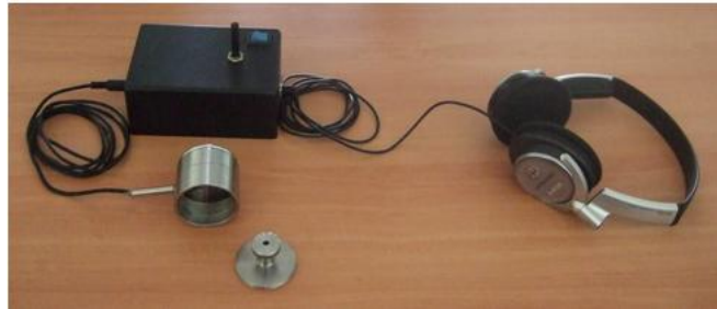
Figure 4.1: Lab prototype of an electronically enhanced stethoscope developed by our group.
