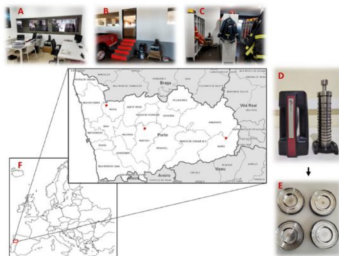
Fig. 1. Sampling campaigns were performed in three microenvironments, A) common area, B) garage, and C) personal protective equipment storage room with a low-pressure impactor (D) over 24 h of a regular working day to collect four fractions of fine (PM 2.5 , and PM 1.56nm ) and ultrafine (PM 54.5nm , and PM 30.8nm ) PM (E) inside three fire stations located in the Porto district (F; North of Portugal).
