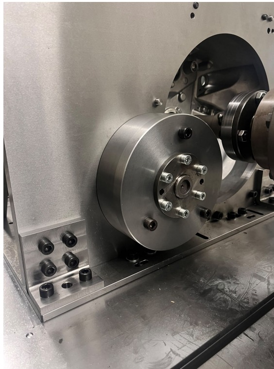
(b) Differential Lock System mounted on the test bench
