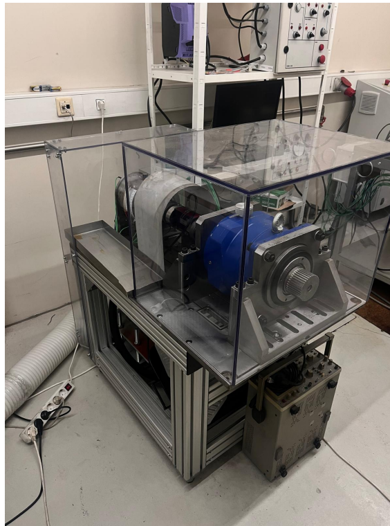
Figure 5.2: No-load power loss test rig
