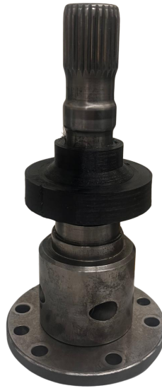
Figure 5.12: 3D-printed seal mounted on the output interface
