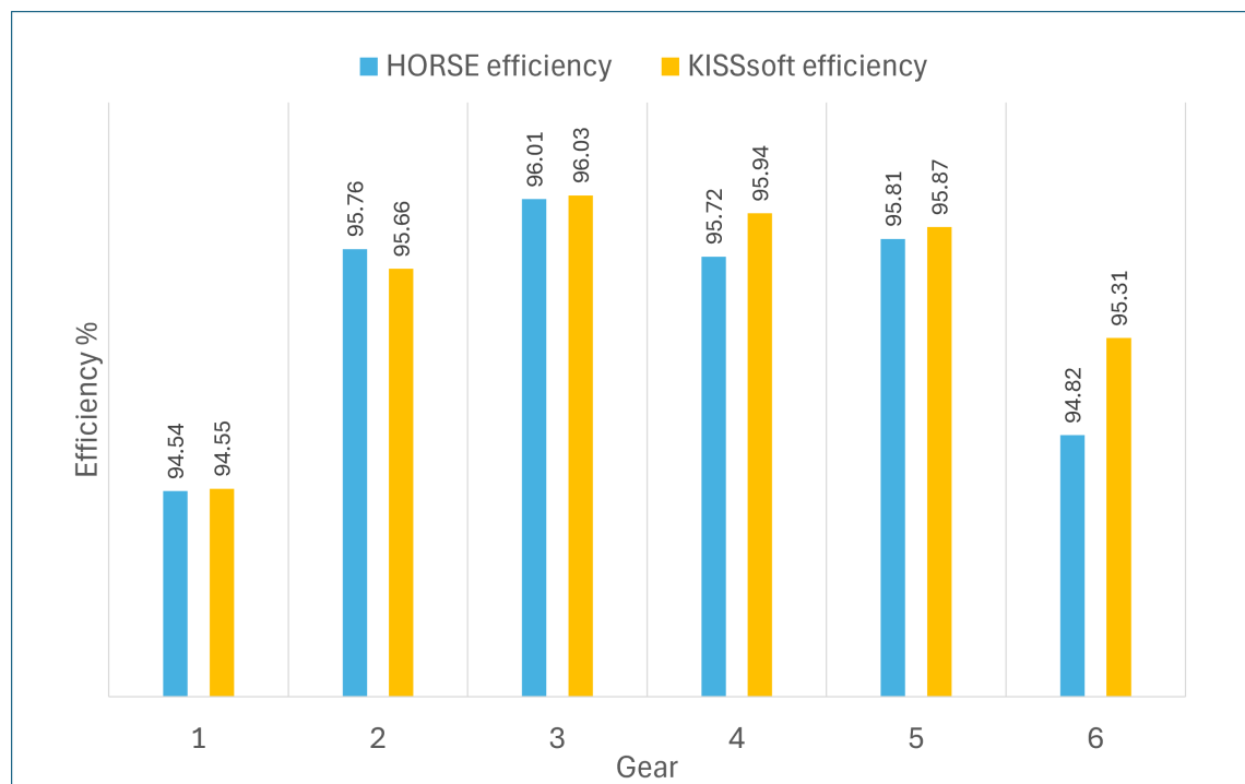
Figure 6.9: Efficiency derived from the tests carried out at HORSE and from the KISSsoft model-Version 2
