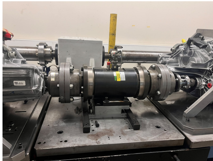
(b) Central sensor assembly mounted on the test bench
