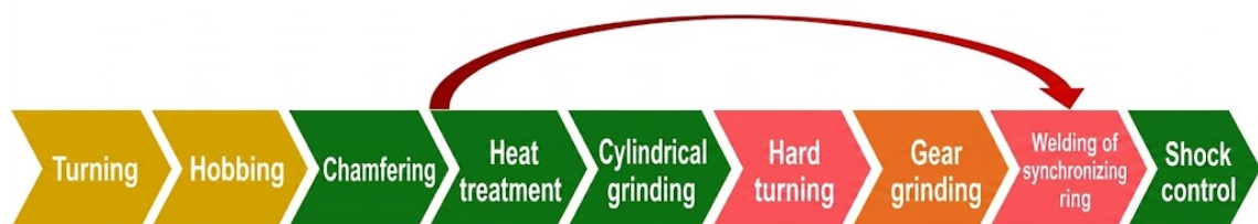
Figure 3.16: Manufacturing line of idle gear of 2 nd Golden version
