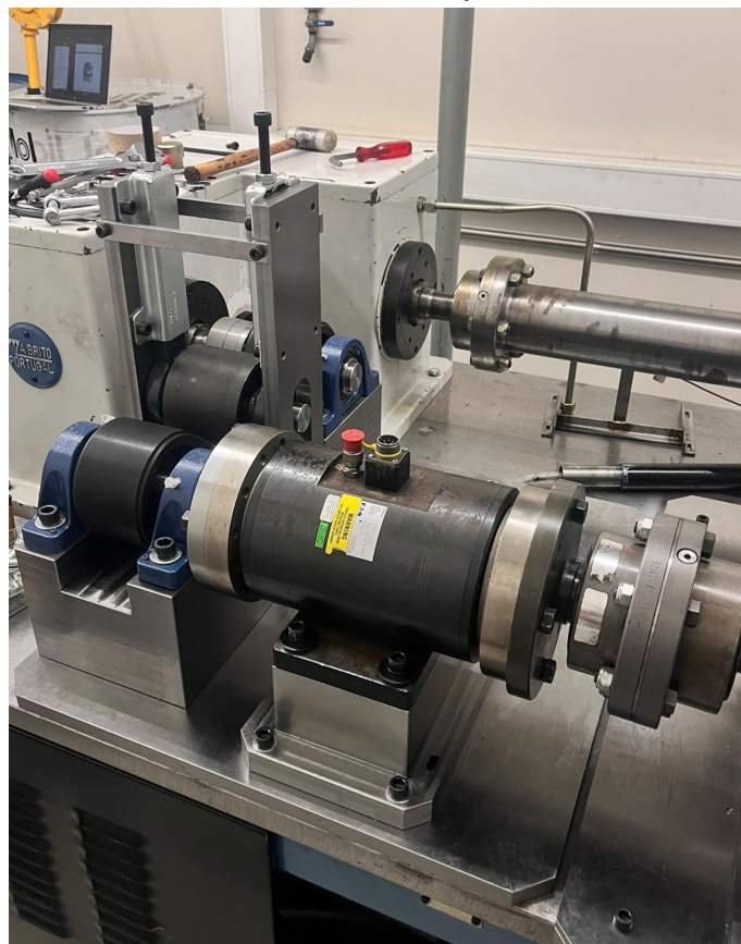
(b) Belt drive assembly mounted on the test bench
