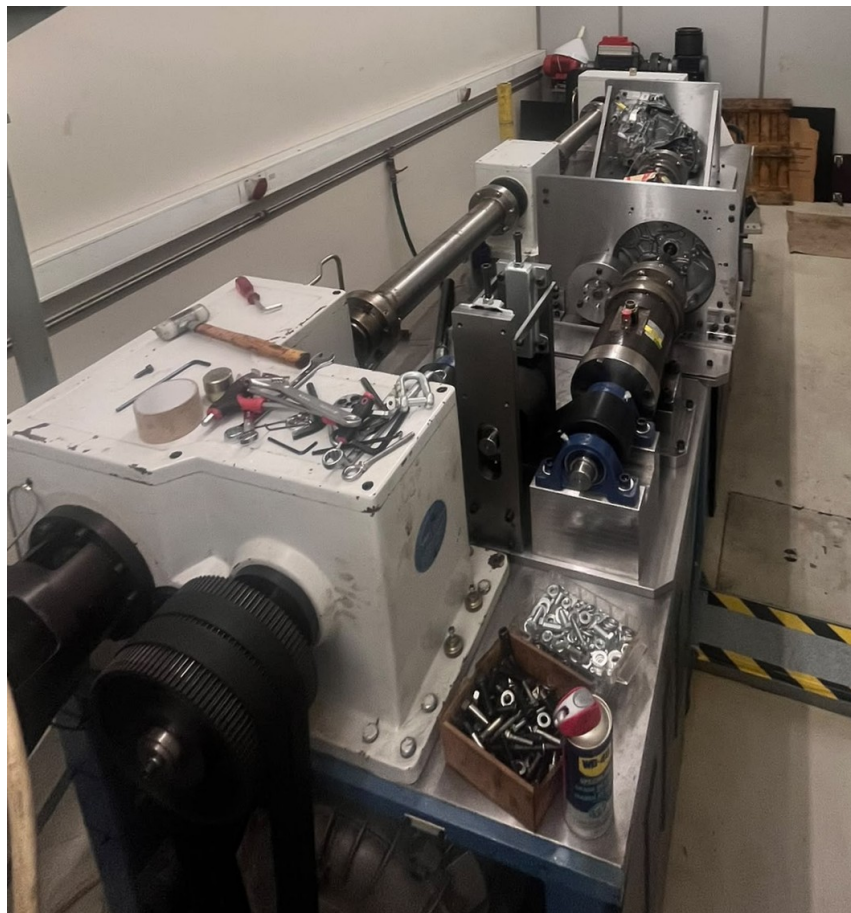
(b) Test bench adapted for the JT4 gearbox
