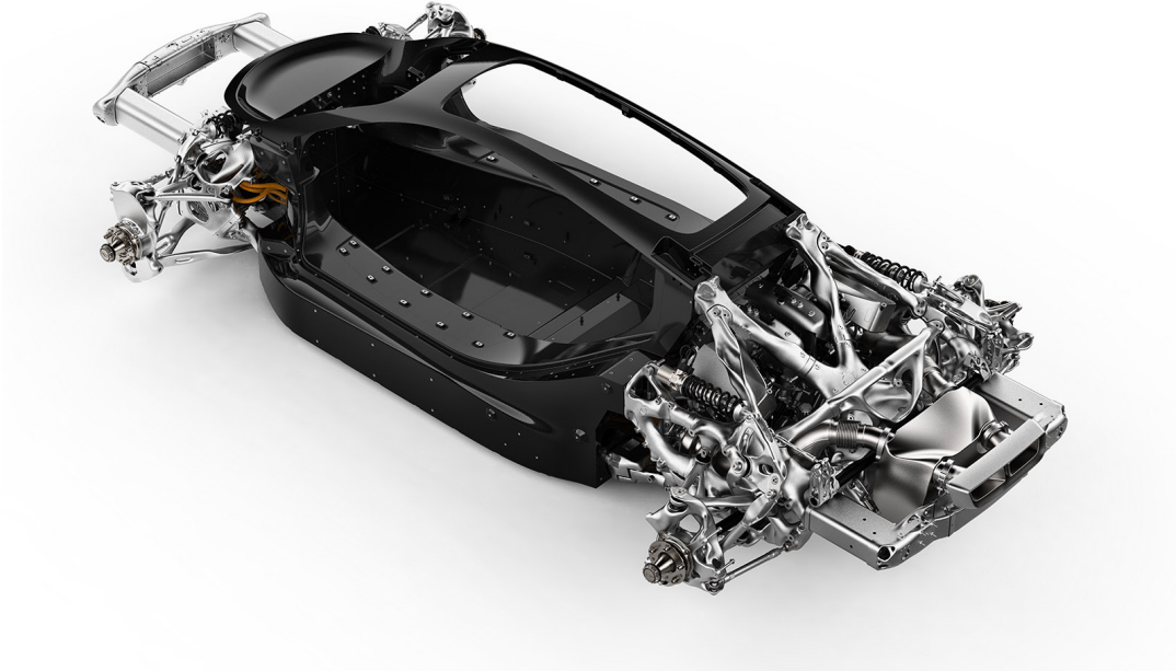
Figure 2.2: The rolling chassis of the Czinger 21C hypercar. The organically shaped metallic nodes that link the front and rear suspension and the powertrain to the central carbon-fibre tub are topology-optimised and produced by metal additive manufacturing through the Divergent Adaptive Production System; their skeletal, bone-like form is the geometric signature of the underlying compliance-driven optimisation. Image: Czinger Vehicles/Divergent, reproduced from Butcher [38].
