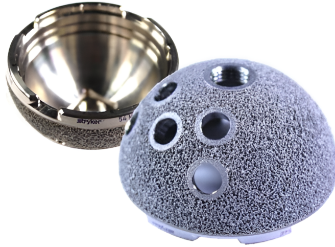
Figure 2.1: A commercially available acetabular cup for total hip replacement (Trident II Tritanium, Stryker), produced from Ti-6Al-4V by laser powder bed fusion. The bone-facing surface carries an integrally printed porous lattice whose interconnected porosity approaches that of trabecular bone, lowering the effective stiffness to limit stress shielding and offering a scaffold for bone ingrowth. Adapted, showing a single design from a larger comparison, under CC BY 4.0 from Dall’Ava et al. [34].
