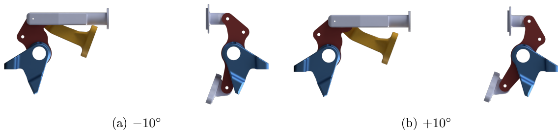
Figure 5.4: The suspension assembly modelled in Autodesk Fusion, shown at the two extremes of the rear axle's roll range, (a) -10^\circ and (b) +10^\circ . The roll-damper bracket is the yellow part. Sweeping the assembly through this range recovers the bracket's motion, identifies how each load is introduced, and generates the clearance envelope that defines the design space.
