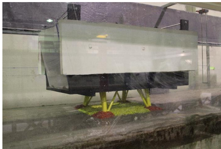
Figure 31 – Hybrid jacket model (small-scale test).
