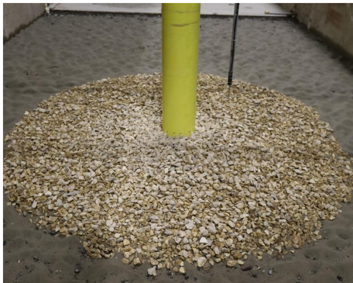
Figure 77 – Static protection after 3000 waves (MS test).
