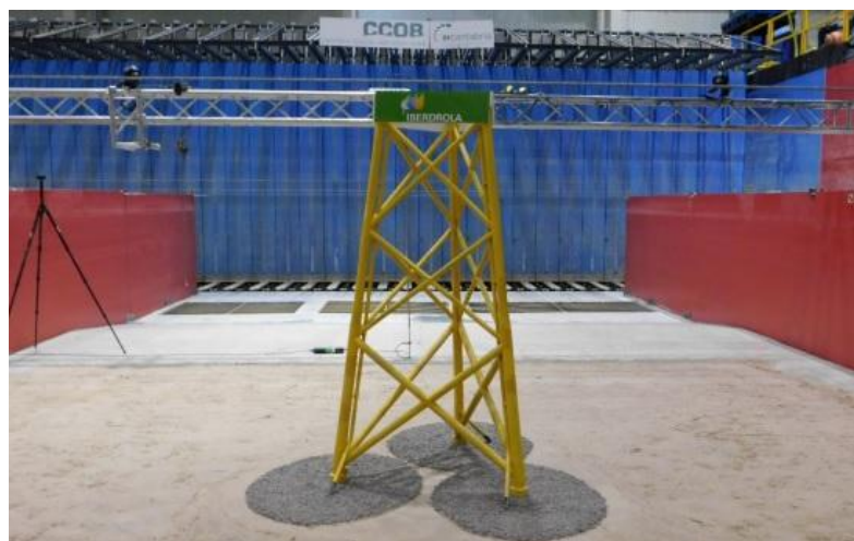
Figure 7 - Scour protection for a model of the East Anglia One 3-leg jacket (Sarmiento et al. , 2021).
