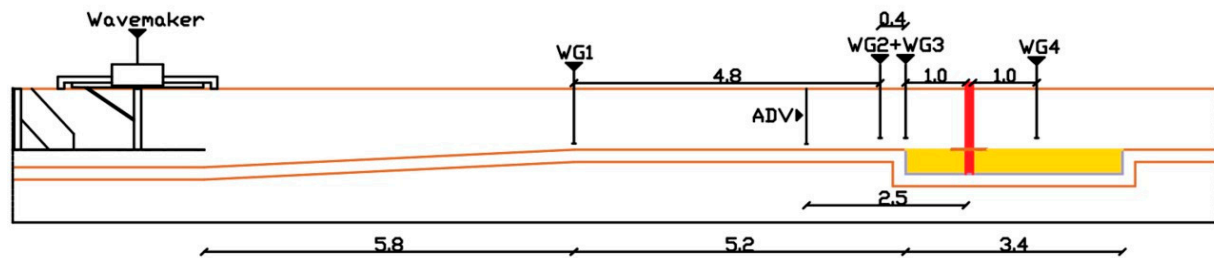
Figure 1. Experimental setup and wave gauge (WG) placement (dimensions in meters).
