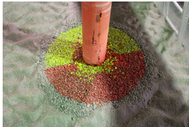
Figure 8. M_WI_14_3000 test scour protection.
