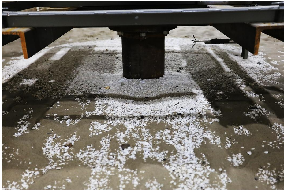
Figure 83 – Dynamic protection deformation after 3000 waves (HMD test).
