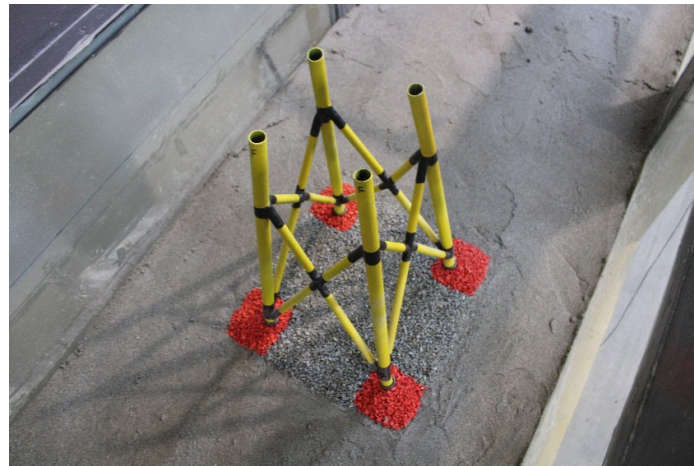
Figure 5. Scour protection for the four-leg jacket model.
