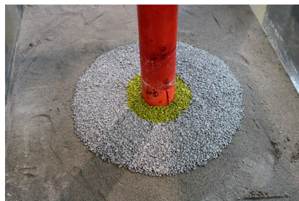
Figure 3. View of the scour protection (with demarcation of the amplification zone).
