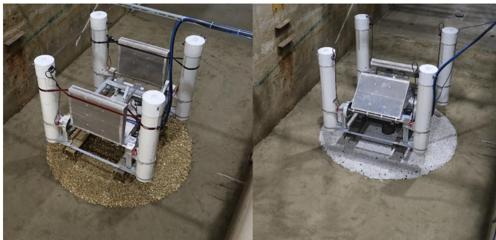
Figure 38 – Large-scale scour protection model for the hybrid structure: static protection (left), dynamic protection (right).
