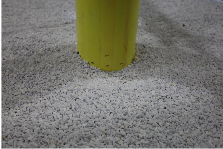
Figure 82 – Dynamic protection deformation after 3000 waves (MD test).
