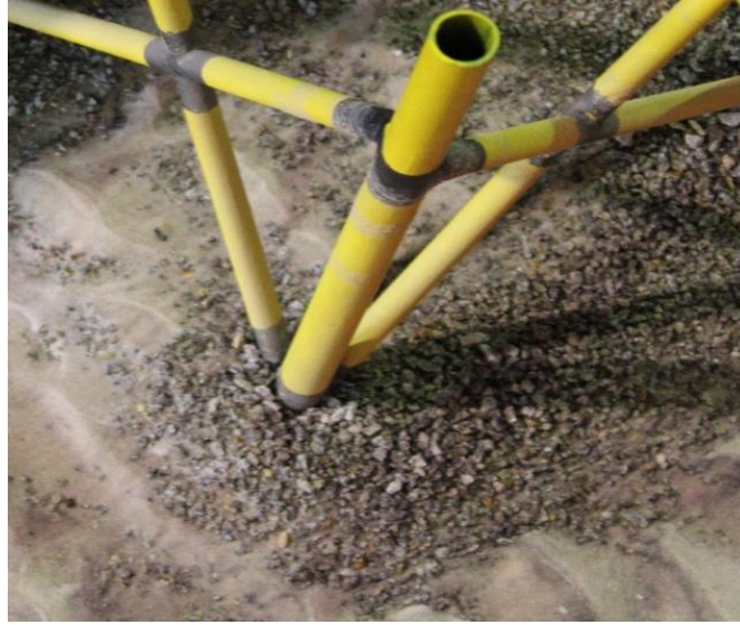
Figure 76 – Pile D after 3000 waves (J_WR_14 test).
