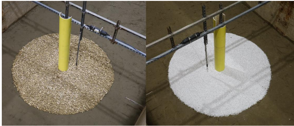
Figure 37 – Large-scale scour protection model for a monopile: static protection (left), dynamic protection (right).
