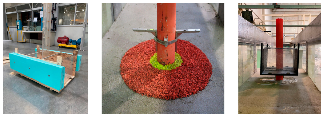
Figure 5. Oscillating surge WEC model construction and installation.
