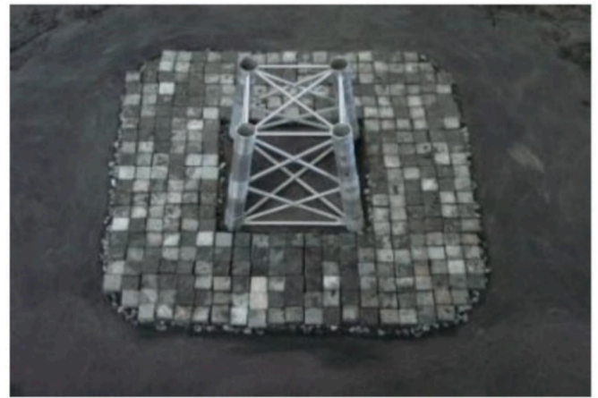
Fig. 12. - Scour protection model for a 4-leg jacket (Hsin-Hung et al., 2014).
