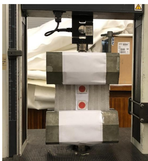
Fig. 5. Apparatus of tensile strength tests of the geosynthetics.
