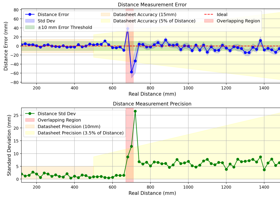
Figure 4.3: Distance measurement error and standard deviation after calibration as functions of the real tested distances. The region marked in red indicates the distance interval with significantly higher error and variability, revealing reduced measurement accuracy and precision in that range.
