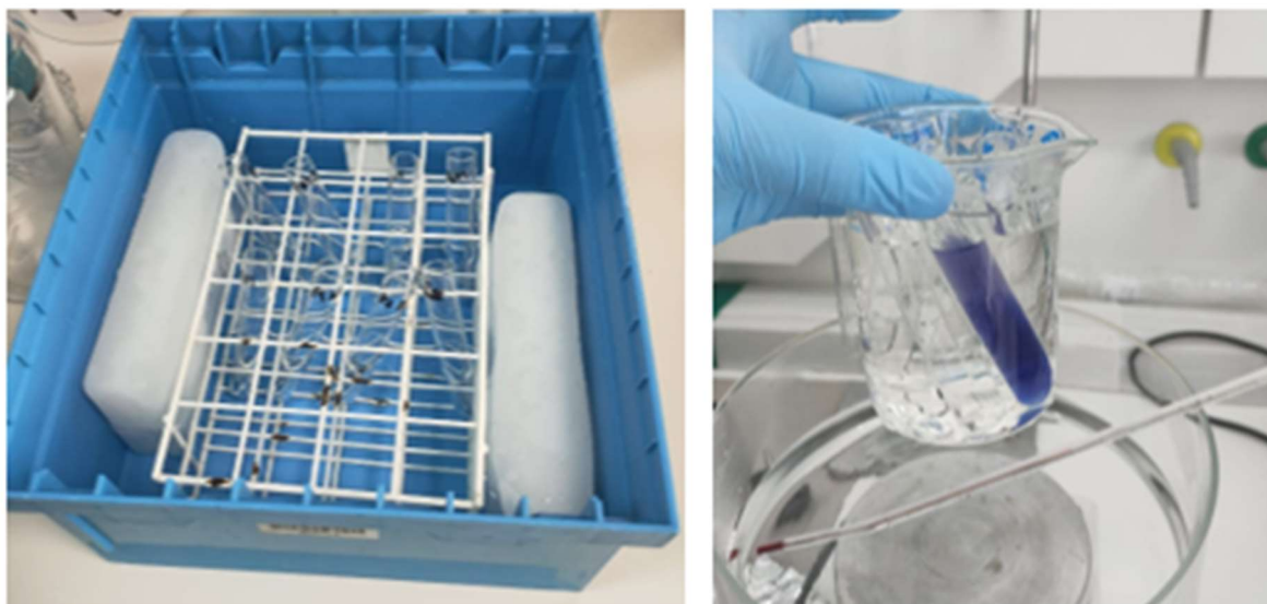
Figure 19 - Methodological setup for the semi-quantitative detection of nitrates: (left) initial low-temperature stabilization phase, showcasing the test tubes arranged chronologically inside the partitioned grid within a controlled ice bath; (right) final reaction phase, where all sample tubes, including the characteristically purple-coloured nitrate reference standard, are consolidated inside a graduated beaker to provide structural support for subsequent immersion in a thermoregulated hot water bath.
