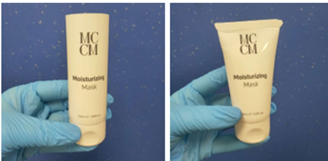
Figure 3 - Primary packaging integrity: Visual comparison of a cosmetic tube before (open) and after the hermetic sealing process.
