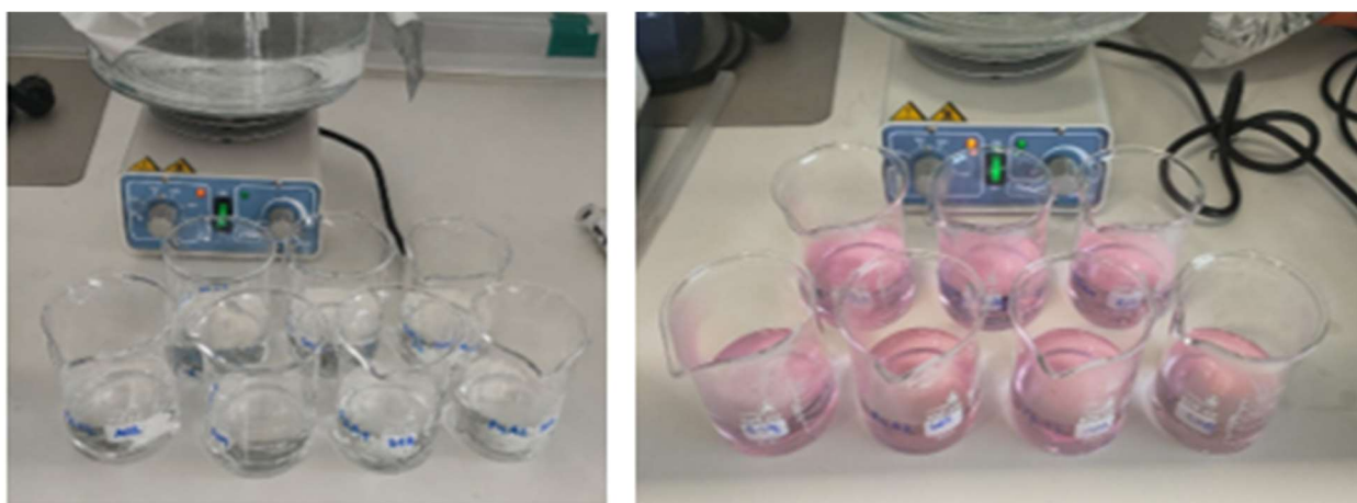
Figure 18 - Determination of oxidisable substances in water samples: colorimetric evaluation based on the potassium permanganate redox reaction, contrasting the initial analytical setup (left) with the qualitative persistence of the pink hue (right) as evidence of compliance with strict pharmacopoeial purity specifications.
