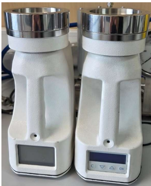
Figure 14 - Environmental biocontamination control: Active air samplers utilized for the quantitative microbiological assessment of airborne viable particles within classified cleanroom environments.
