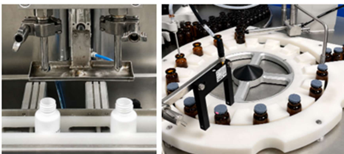
Figure 2 - Automated primary packaging equipment in an ISO 8 cleanroom: (left) Liquids filling machine; (right) Vials filling machine;
