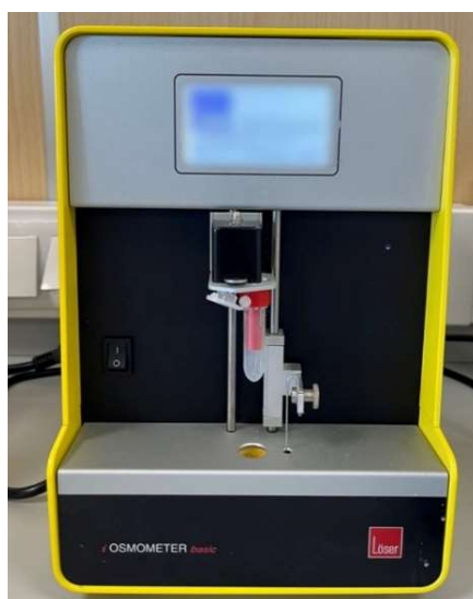
Figure 11 - Cryoscopic osmolality determination: Löser type 7 osmometer utilized for the precise tonicity assessment of sterile mesotherapy and mucosal formulations.
