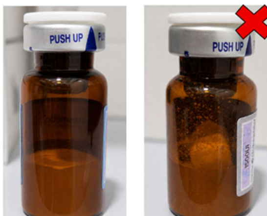
Figure 15 - Macroscopic evaluation of lyophilised morphology: Comparison between a fully compliant, intact, and porous (left) and a rejected unit exhibiting structural collapse and melt-back (right).
