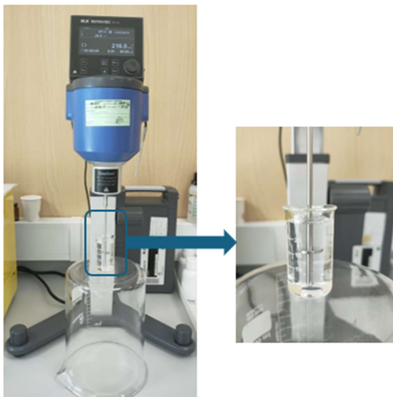
Figure 10 - Rheological quality control: IKA Rotavisc lo-vi relative needle viscometer employed for the routine viscosity assessment of semi-solid cosmetic batches.
