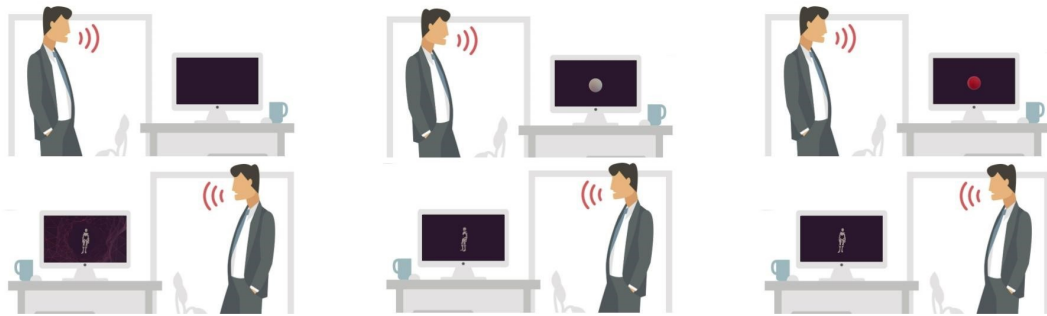
Figure 7.6: Voice-command interaction workflow in A Máquina Sensível . The user issues spoken commands that are transcribed through the speech recognition module and mapped to scene operations, enabling the real-time creation and transformation of virtual objects (e.g., spheres, humanoid figures, and color modifications).
