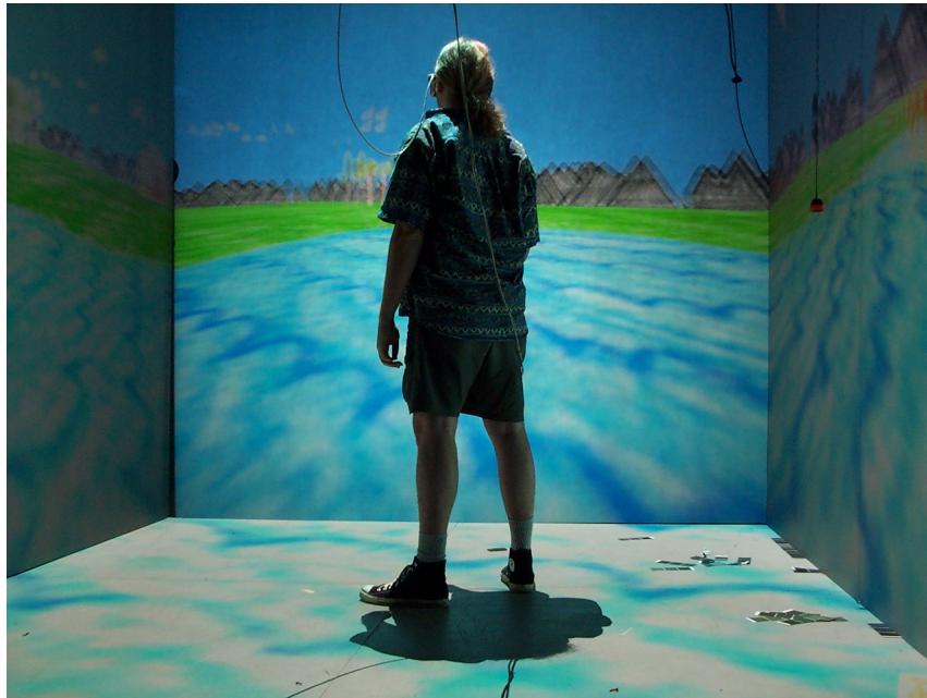
Figure 1.1: The Cave Automatic Virtual Environment (CAVE) at the Electronic Visualization Laboratory (EVL), University of Illinois at Chicago. Photograph by Dave Pape (self-timed capture), Public Domain, via Wikimedia Commons: https://commons.wikimedia.org/w/index.php?curid=868395 .
