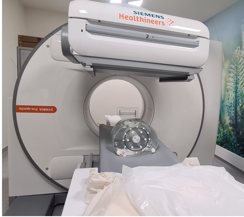
Figure 3.4: Symbia Pro.specta setup for the acquisition of the NEMA phantom.
