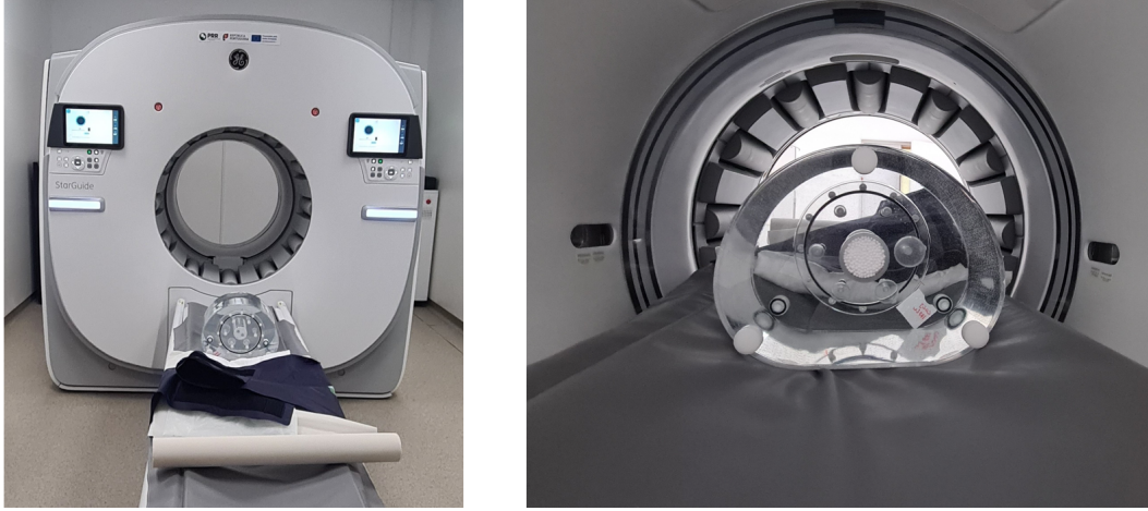
Figure 3.2: StarGuide setup for the acquisition of the NEMA phantom (left) and a close-up view of the NEMA phantom positioned inside the scanner bore (right).
