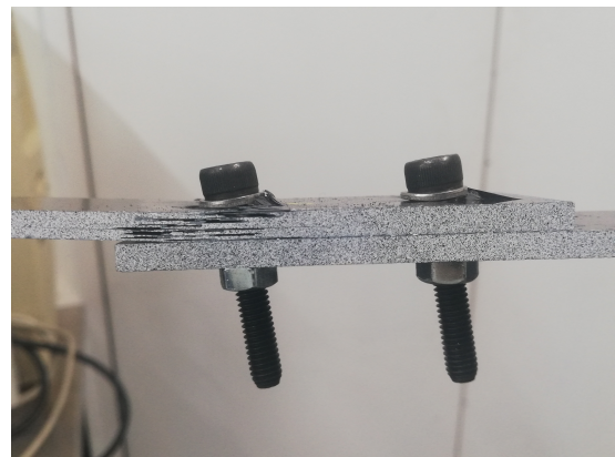
(b) Side view showing delamination
