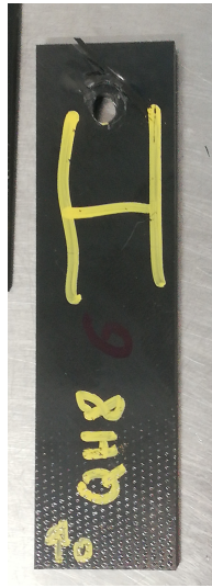
(a) QH specimen after bearing test.
