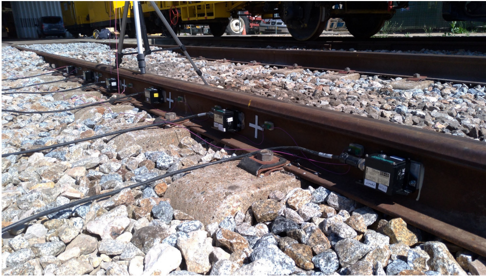
Figure 2.6: Examples of on-site instrumentation: accelerometers (black boxes) plus active and passive targets for a vision-based system to measure track deflections.
