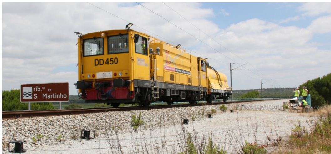
Figure 3.11: Monitoring vehicle used to validate the COURSE system prototype.
