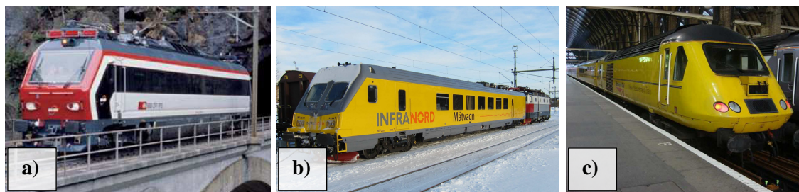
Figure 2.9: (a) the Swiss SBB monitoring vehicle, (b) the Swedish Infranord monitoring vehicle, and (c) the UK Network Rail New Measurement Train (adapted from Rivas, 2013).
