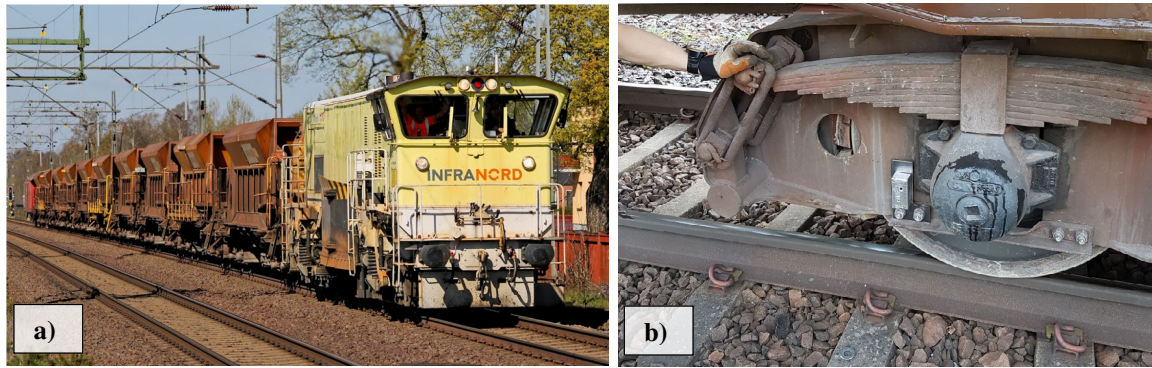
Figure 2.20: (a) Instrumented railway vehicle used in Björklind's experimental campaigns, and (b) position of one accelerometer on the vehicle's bogie (Björklind, 2018).
