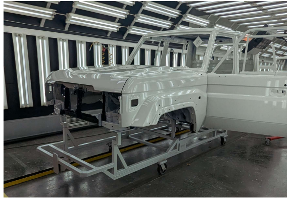
Figure 3.26: Quality control top-coat inspection post (QCT1)
