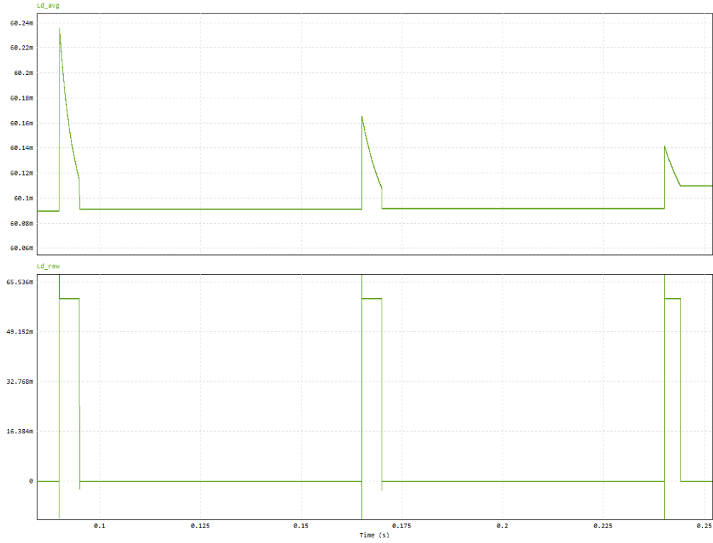
Figure 4.10: Instantaneous and averaged inductance estimation. The averaged value converges to a stable result despite transient spikes.
