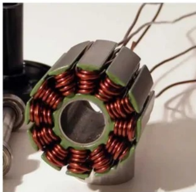
Figure 2.3: [11]Side-by-side comparison of concentrated (left) and distributed (right) stator windings. Concentrated windings place each coil around a single tooth, while distributed windings span multiple slots. The corresponding back-EMF waveforms for these winding types are shown in Fig. 2.1.
