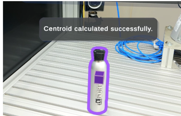
(b) Corresponding XR overlay, where the target object is highlighted and the centroid calculation is reported to the operator.
