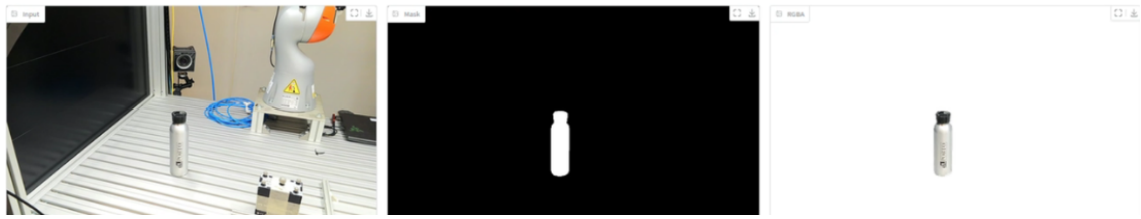
(a) Selected RGB frame, binary segmentation mask, and cropped object representation generated on the edge side.
