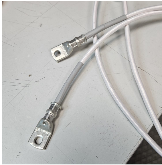
Figure 6.6: Completed termination of a coil.
