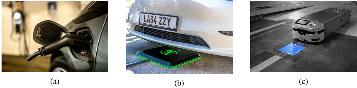
Figure 1.2: Comparison of charging methods: (a) conventional wired charging, (b) wireless IPT for EV parking, (c) wireless IPT for AGVs in industrial settings.
