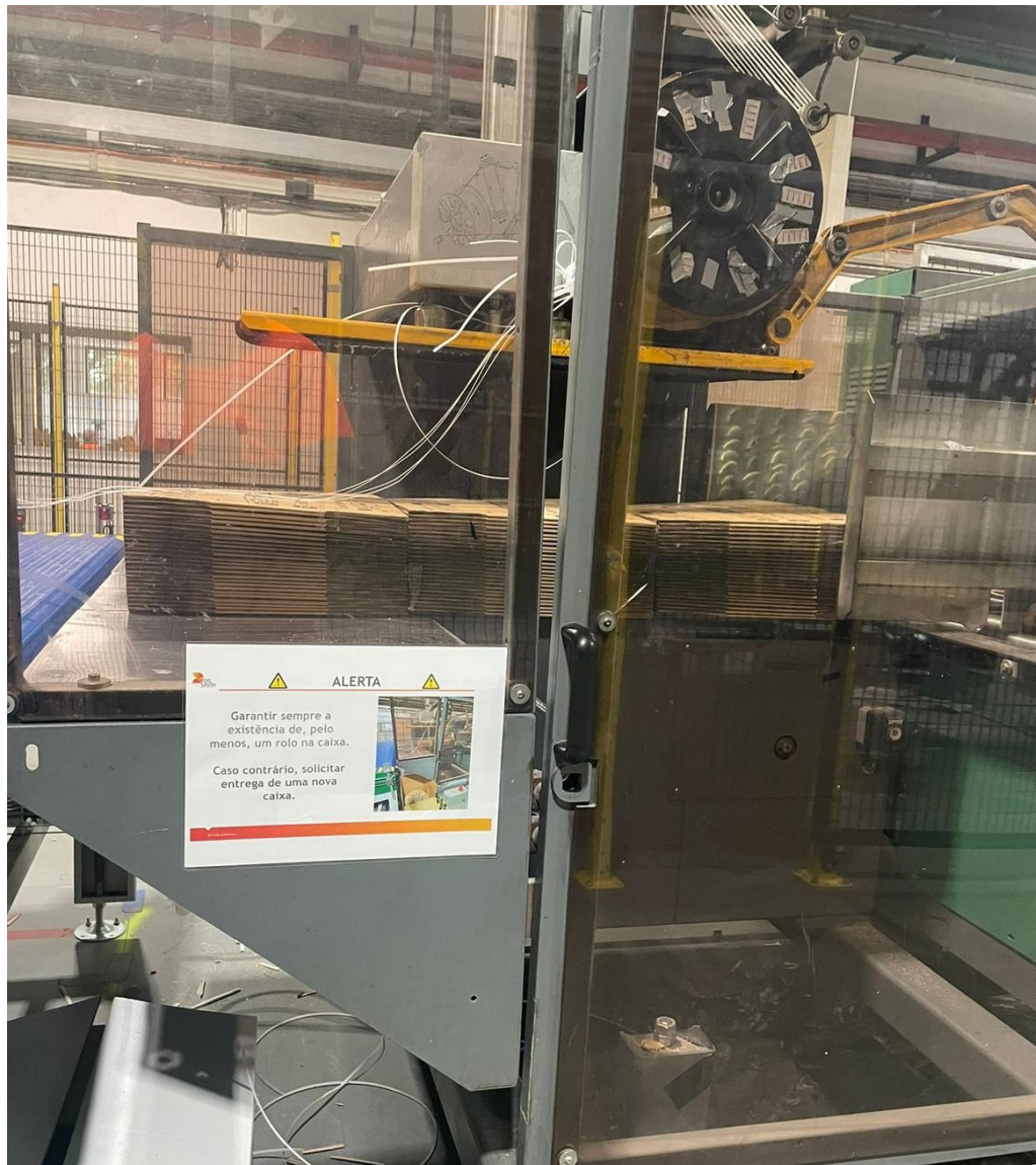
Figure 46: Sign instructing operators to request more strapping band.
