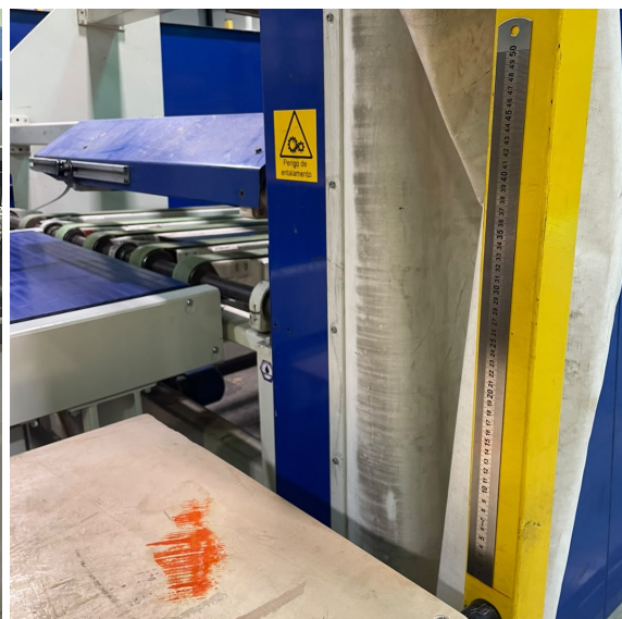
Figure 24: Recording sheet for doctor blade re- Figure 25: Graduated scales installed at the placement and ink tray cleaning. strapping machine.
