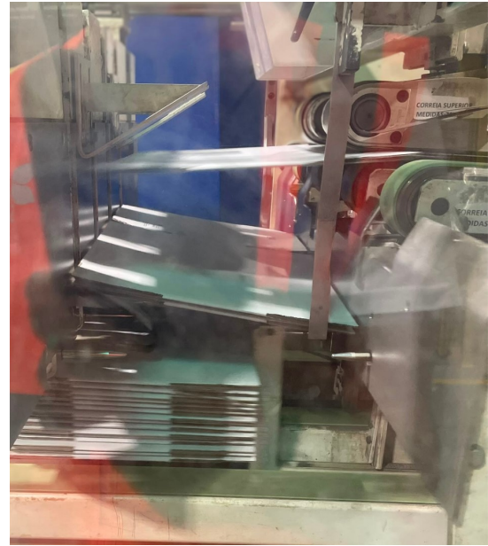
Figure 33: Final state - Counter stacker.
