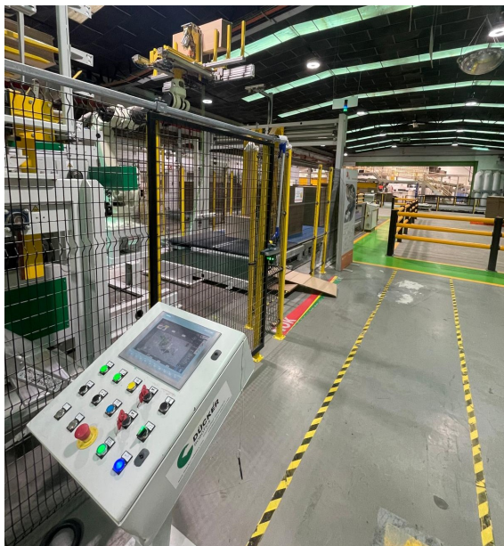
Figure 36: Pre-feeder control system.
