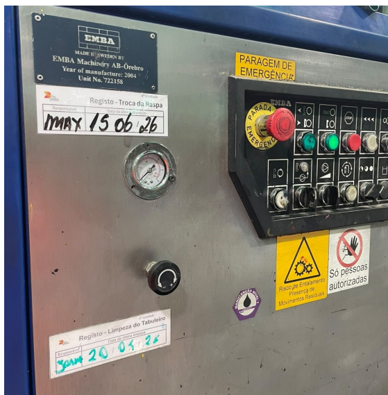
Figure 24: Recording sheet for doctor blade re- Figure 25: Graduated scales installed at the placement and ink tray cleaning. strapping machine.
