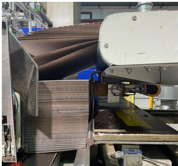
Figure 31: Component responsible for sheet alignment, after adjustment.
