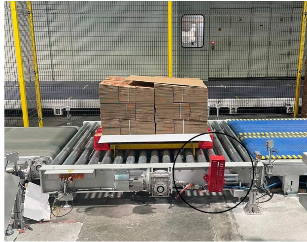
Figure 35: Protective cover fitted to the pallet detection photocell.
