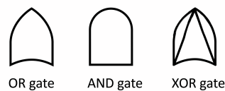
Figure 2.5: Fault tree logic gate symbols. Adapted from: (Kabir, 2017)
