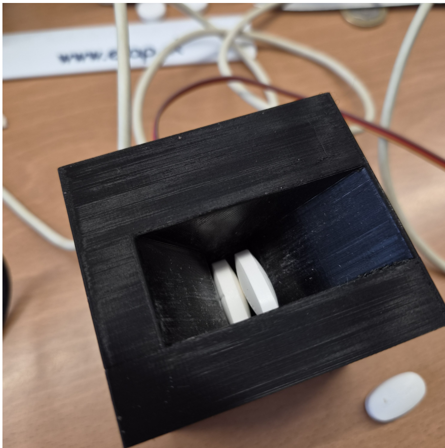
Figure 4.7: Example of a jam in the Ben-u-ron 1000 mg compartment: a tablet in the undesired orientation, with a second tablet partially occupying the remaining space, blocking rotation.
