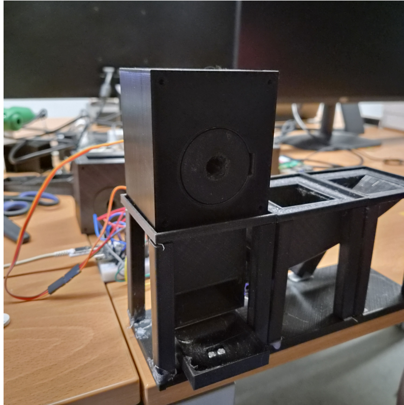
Figure 4.4: Dispensing test scenario: servo cylinder assembly, funnel, and final platform with rigidly mounted load cell, used across the 50 dispensing cycles of Phase 3.
