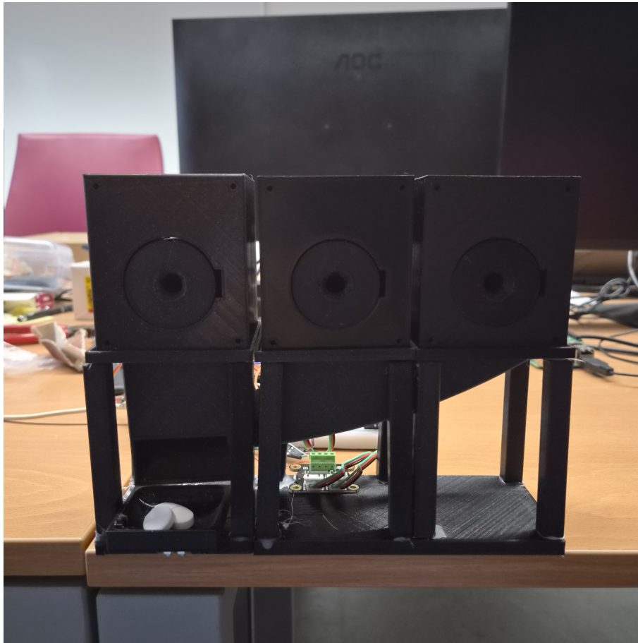
Figure 3.1: The final, three-compartment MedBox prototype: rotating-cylinder dispensing mechanism, shared collection platform with load cell, and control electronics.
