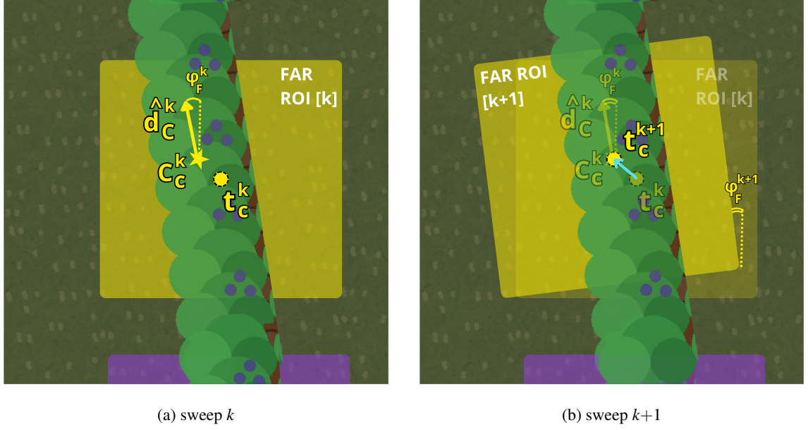
Figure 5.6: Predictive placement of the FAR region across two consecutive sweeps: the box is centred on the FAR centroid from the previous sweep and re-projected along its direction to hold the fixed separation L from the CLOSE centroid.
