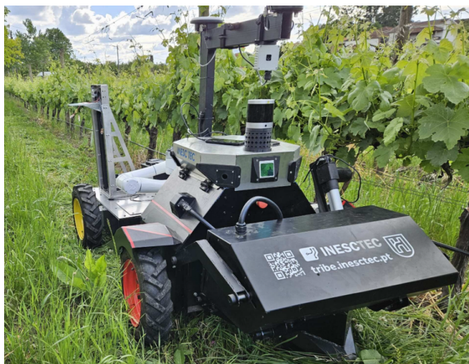
Figure 4.2: The Modular_E robotic platform used for real-vineyard data collection and deployment
