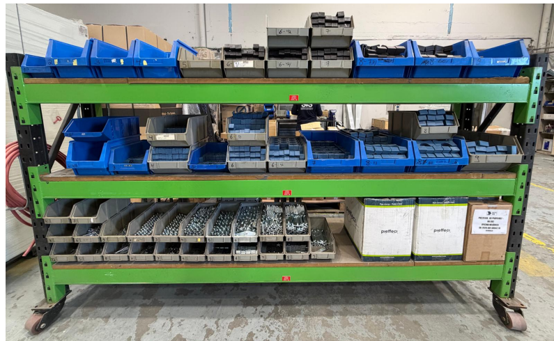
Figure 4.9: Implemented centralised pipe clamps storage
