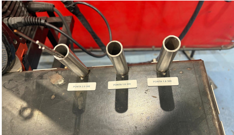
Figure 4.14: Fabricated support for electrode stubs
