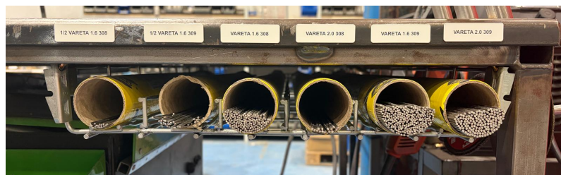
Figure 4.13: Custom wire rack for welding electrodes
