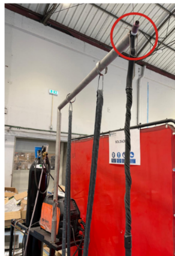
Figure 4.17: Vertical support for the welding torch
