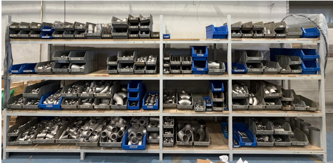
Figure 4.8: Centralised storage of pipe fittings - physical implementation
