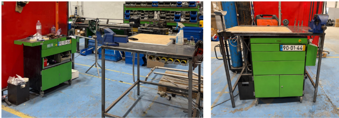
Figure 4.20: Before and after of the welder's tool cart positioning
