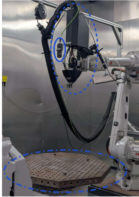
Figure 3.1: Overview of the experimental DED cell featuring an ABB IRB4600 robot. The camera mounted on the end-effector is highlighted with a solid circle, the printing table with a dash-dot circle, and the WLAM system with a dashed circle.
