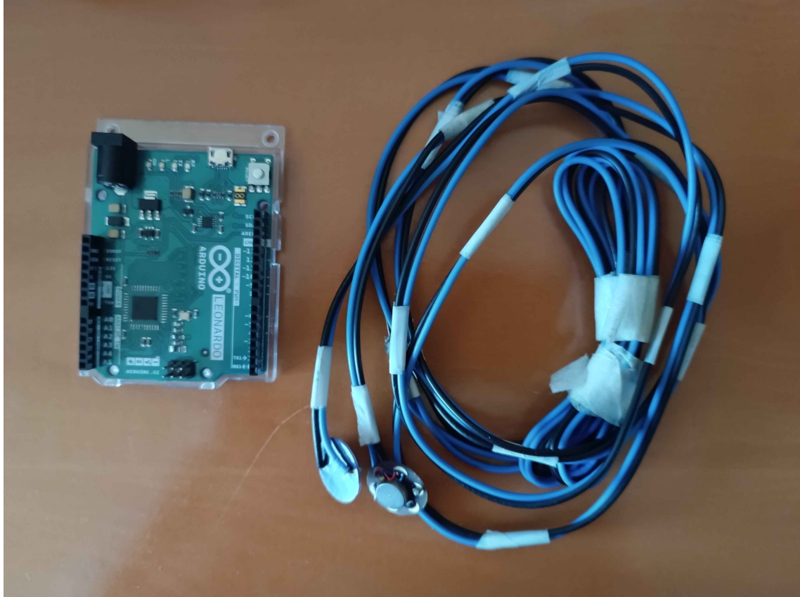
Figure 3.6: Arduino Board and Vibration Motors Used in the Project
