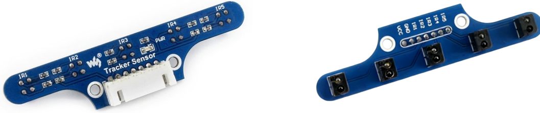
(a) Top view showing the interface connector.
