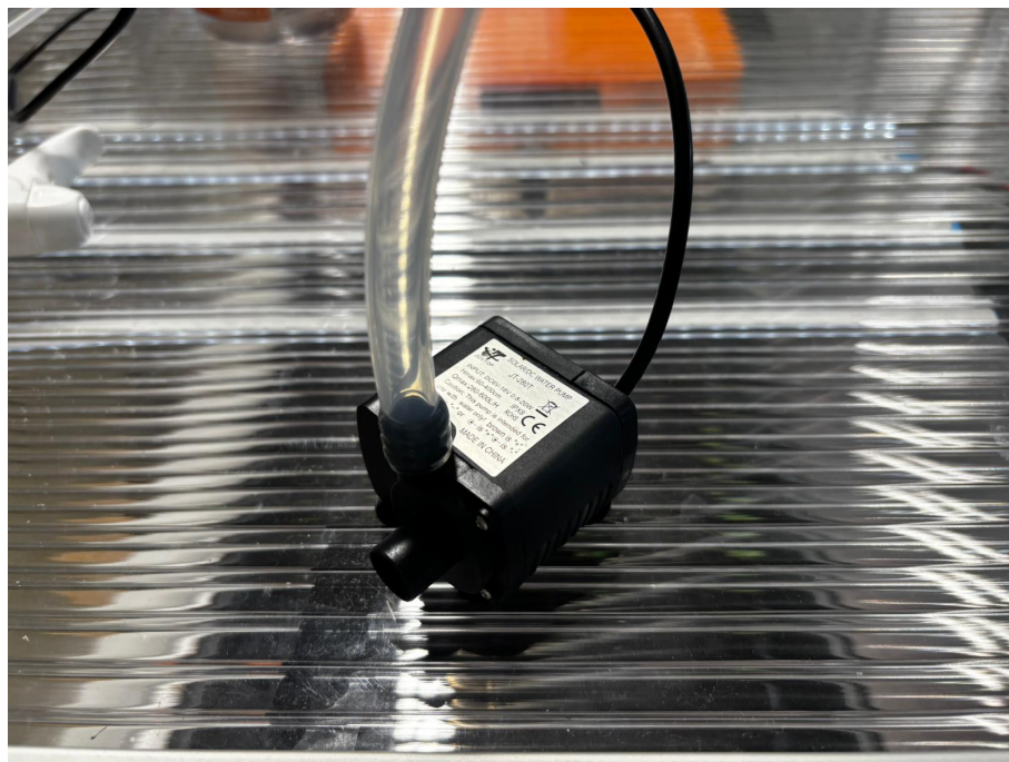
Figure 5.10: JOVTOP JT-280T submersible brushless DC water pump.
