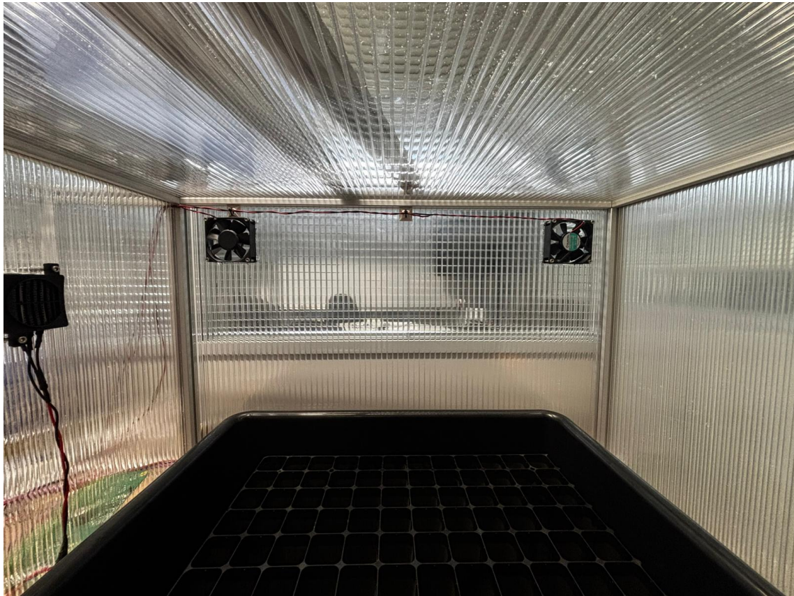
Figure 8.2: Interior view of the VineComputer growing chamber showing the two Sunon KDE1208PTS1 axial fans installed at the upper corners of the rear wall.
